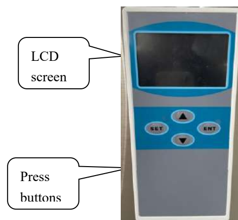
Pic. 2 Control board
