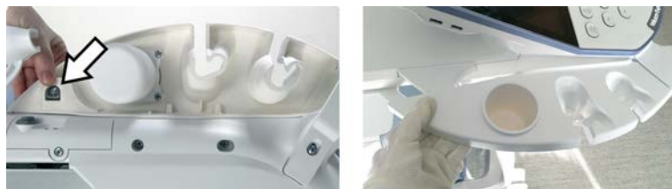
Figure 2-9 Removal of the basic version of the left and right Probe Holder inserts. For installation, just push them back on the user interface until you hear a "click" noise.
