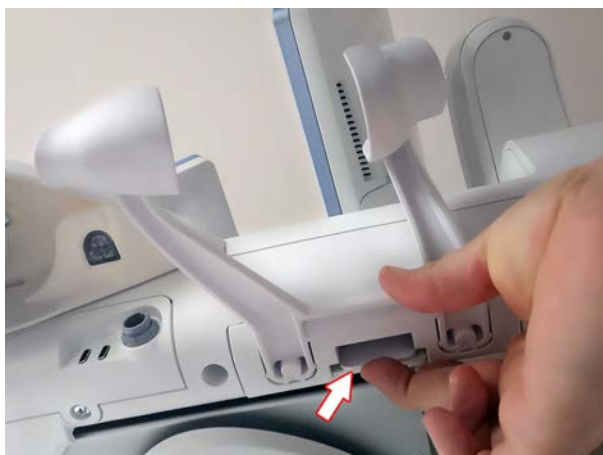
Figure 2-11 Removal of the left and right Endocavity probe holders. For installation, just push them back into the user interface until you hear a “click” noise.
