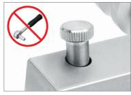
Blades can be replaced without any tool, using the knurled screws.
