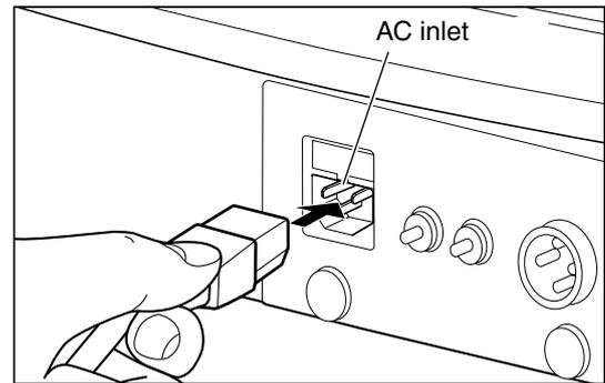
The AC power indicator is lit and the in built batteries will begin to automatically charge. After Battery 1 has been recharged, recharging of Battery 2 (option) starts automatically.
