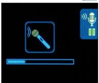
A patient data recording feature (microphone symbol) is active on the recorder to allow a voice recording of patient data. Voice recordings can be played back within DARWIN2, and the details can be typed in using DARWIN2 later.
