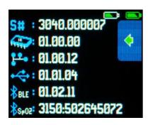
This menu displays specific recorder information, including the version and serial numbers of the recorder and other attached Bluetooth® devices/accessories. This information must be available when contacting Schiller service departments for help and troubleshooting.
