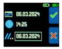
3. After completing the last adjustment, press the UPPER button to Save or the LOWER button to Cancel.
