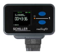
If not disabled in the configuration, the recorder's orange LED (1) flashes every 5 seconds, indicating the unit is in recording mode.
