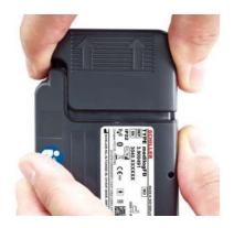
Remove/replace the external battery as follows:
