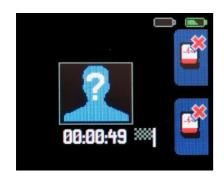
If the recorder detects a recording saved on the memory card that has not yet been read by the PC (not transferred to DARWIN2, false start, mistake), the recording information is displayed when the memory card is inserted as shown. The recording can be deleted by pressing both recorder front panel buttons for several seconds until the full progress bar indicates the recording has been deleted.
