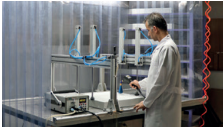
HEPA / ULPA Filter Test System - HF-SCAN 3004
