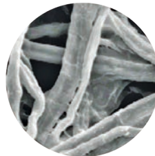
Cellulose Fiber at x500 Magnification
