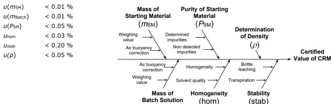
The combined standard uncertainty is calculated by combination of the standard uncertainties of the input estimates according to Eurachem/CITAC Guide "Quantifying Uncertainty in Analytical Measurement" and ISO 17034.[2][5]
