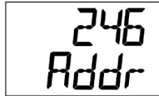
2 Screen: Modbus address
