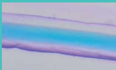
Microscopic image of BMG fibre stained with coloured dyes, demonstrating core shell structure.
