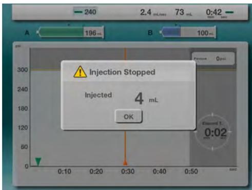
If the Stop button is pressed during an injection, the injection will stop.
