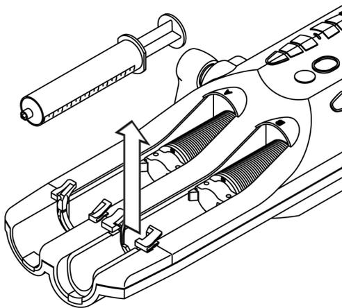
After aligning the syringe lift upwards and remove the syringe from the syringe pocket.
