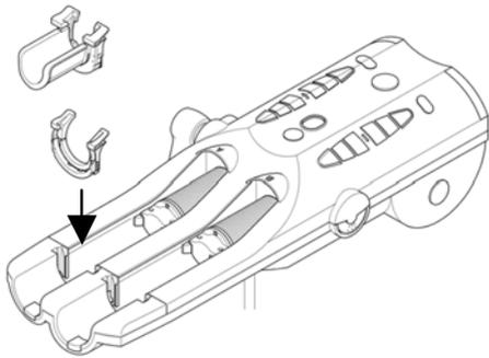
The syringe adapters of the DUAL SHOT alpha7 insert into the Powerhead identically regardless of whether it's a 200mL or 100mL adapter. The adapter simply slides into the Powerhead syringe pocket.
