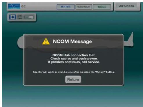
When an abnormality exists between the Console and the NCOM Hub, the message on the left is displayed.
