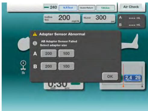
In the event a syringe adapter is not installed or detected, a manual selection window will appear. Depending upon the type of protocol the option for the A-side or both sides will be presented.
