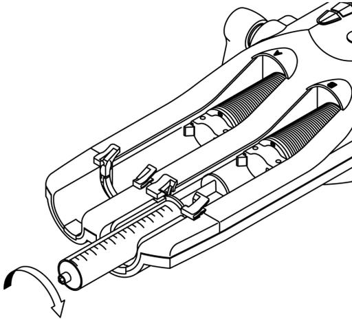
The syringe must be aligned and pushed into the slot of the adapter for proper insertion. Proper alignment consists of aligning the flat sides of the syringe with the adapter slots and ensuring the syringe notch is pointing upwards.
