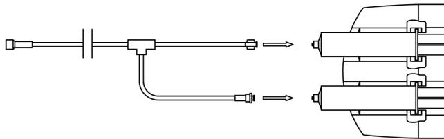
Connect the injection line to the syringe.
