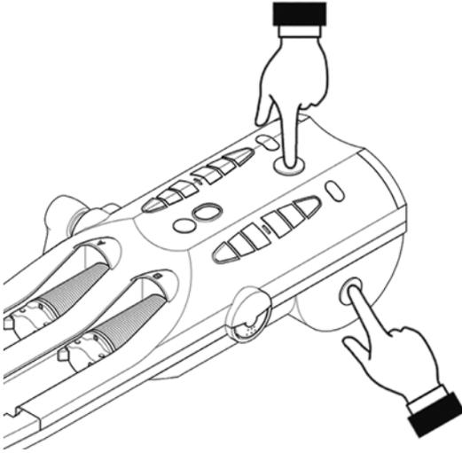
Injection stop buttons are located on both sides and atop the Powerhead.
