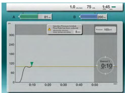
If the injection pressure reaches the pressure limit setting, the pressure limit function will activate and reduce the flow rate until the injection pressure is maintained at the pressure limit setting.
