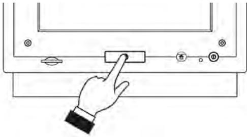
Pressing the "Stop" button on the Console during an injection stops the injection.
