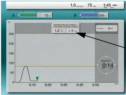
During an injection a screen similar to the one on the left will be displayed. A real-time pressure graph will be shown during the injection.
