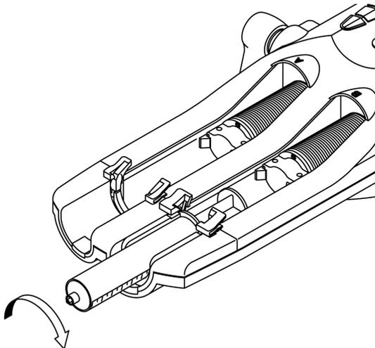
To remove the syringe from the adapter, first rotate the syringe either clockwise or counter-clockwise until the flat sides of the syringe are aligned with the adapter.
