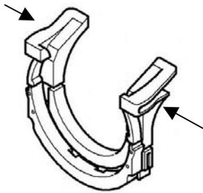
To remove a syringe adapter, squeeze the adapter in the direction of the arrows as shown in the diagram on the left. After squeezing inward, lift the adapter from the syringe pocket area of the Powerhead.
