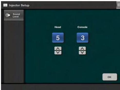
The sound level for the Console (display) or Powerhead (head) can be set independently. Use the  and  keys to set the desired volume.
