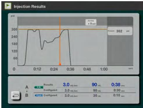
3) The pressure graph displays the pressure values throughout the injection protocol.
