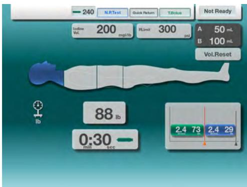
After the user confirms no air is present in the system, it is still possible conditions are not sufficient for the injection to start. If "Air Check" has been pressed, but the injection cannot be performed, a "Not Ready" state will be presented to the user. The "Not Ready" state appears as a blinking "Not Ready" in the upper right corner of the display.
