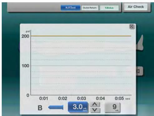
Pressing the N.P.Test key (without an injection first selected) will cause the Needle Placement Test pop-up window to appear. The NPT is available anytime saline is available.
