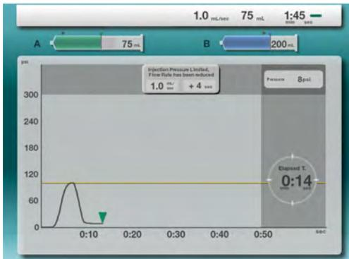
When the injection is completed, the warning message popup will reappear to notify the user the pressure limit was activated during this injection.
