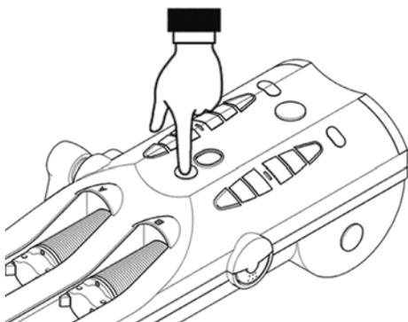
Inspect syringe(s) and tubing to verify that air has been removed. To confirm to the injector that you have removed air, press the Air Check button on the Powerhead.
