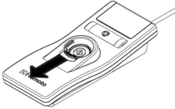
Position the Switch Box as shown, then slide the Start Button cover in the direction shown by the arrow.
