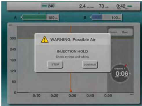
A low pressure monitoring system is designed in the injector for the A-side and B-sides. The message at the left will be displayed when a low pressure condition exists. Low pressure sensing aids in detecting an empty syringe. Refer to the following table for understanding when a low pressure condition exists.
