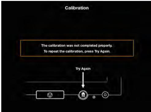
Press the "HOME" button of the console to perform the calibration one more time after the following screen is displayed.
