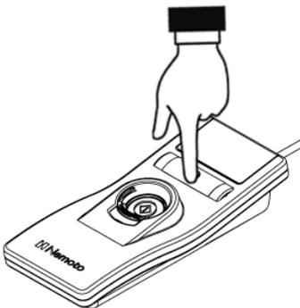
Pressing the Switch Box stop button stops the injection.
