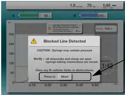
If the injection is stopped due to a blocked line condition the message on the left will be displayed.
