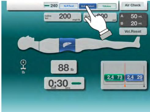
Touch the syringe icon "Quick Return" to access the set-up screen.
