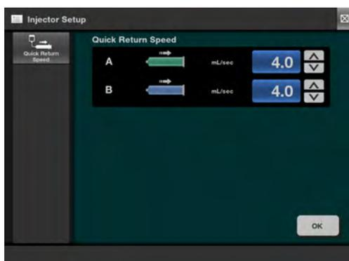
The Quick Return Speed Set determines the speed that will be used to fill the syringes when using the Quick Return (Auto-Return) sequence.
