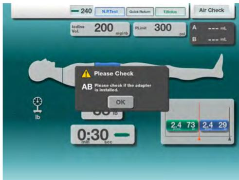
If the Check Air button is pressed and a syringe adapter is not detected or properly installed the message at the left will appear.
