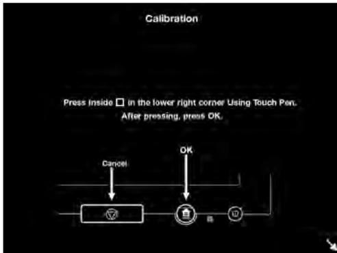
After the following screen is displayed, touch the inside of the red square in the lower right corner with the touch pen.
