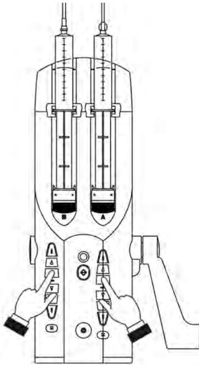
Using the techniques described in the "Connection of the injection line" section purge and remove air from the syringes and tubing.
