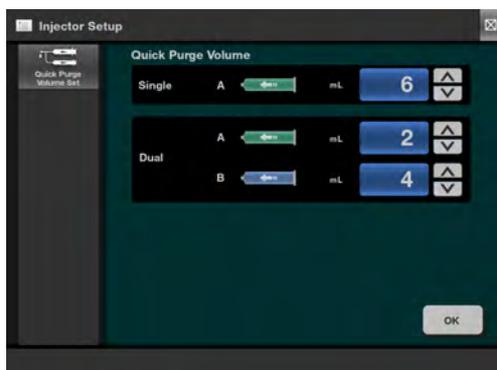
The Quick Purge Volume Set sets the default values for the Quick Purge feature. The Single section sets the default purge volume when only the A-side is being used in the injection protocol.
