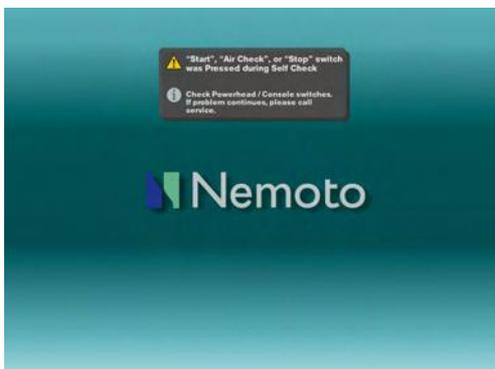
During power up, if any button on the Powerhead, Console, or Switch Box is pressed an alarm message is generated. When the cause of the alarm is corrected, the setup screen will appear without cycling power.
