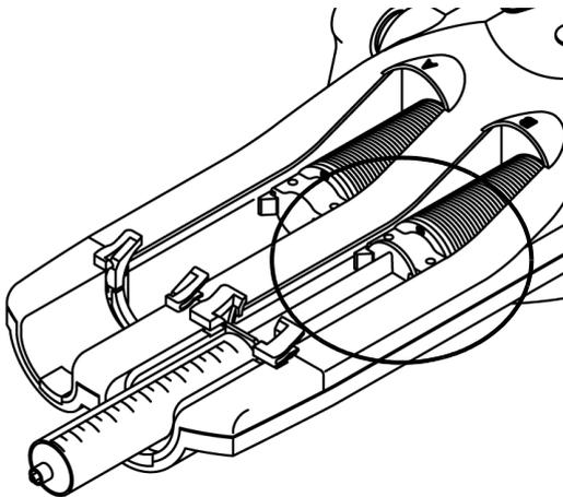
Securely lock the ram clammer onto the syringe plunger. Closely contact the ram with the flange of the plunger.
