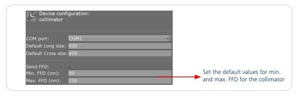
Figure 57. Default settings for collimator
