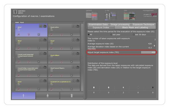
Figure 97. Tab "Exposure Index" with statistical overview
