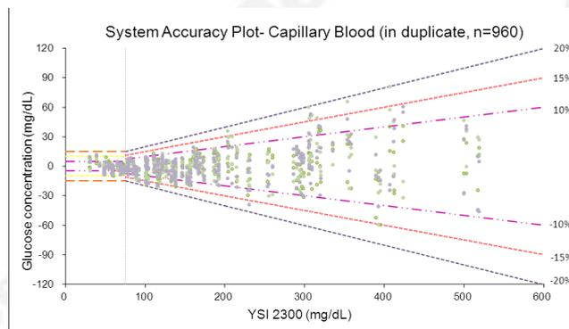
Figure 2 System accuracy plot. Measurement bias of capillary blood glucose obtained with blood glucose monitoring systems versus the laboratory reference device of Yellow Spring Instrument 2300. The lines represent  $\pm 15$ mg/dL (0.83mmol/L) for glucose concentrations  $< 100$ mg/dL (5.5mmol/L) and  $\pm 15\%$  for glucose concentration  $\geq 100$ mg/dL (5.5mmol/L).
