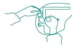
7 Tighten excess material around eyepieces. Just before procedure remove top.
