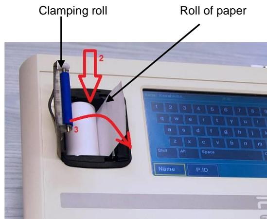
If there is any irregularity caused by jammed paper, do out; open the lid, take the paper out, cut the crumpled clamping roll and install the paper properly.
