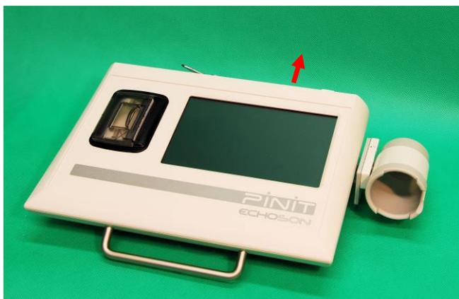
3) Carefully put the upper part of housing on the top side
