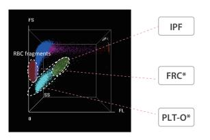
In ERP channel, PLT-O\* can prevent the interferences of Fragmented Red Cells(FRC\*) and offer more accurate PLT count compared to traditional technology. IPF measures the Immature Platelet Fraction, which can be used to reflect thrombopoiesis capabilities of patients.
