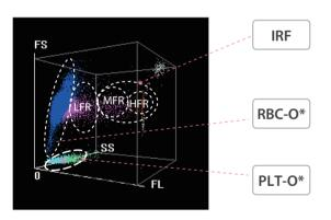
With the SF Cube cell analysis technology, Reticulocytes are differentiated from the other red cells by their reaction with fluorescent stain. Besides the traditional parameters such as RET# and RET%, BC-6800Plus provides data concerning immature reticulocytes (IRF), which can assist in early diagnosis of anemia and monitoring the bone marrow response to therapy.
