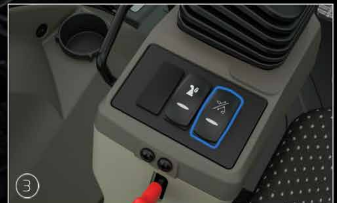
Shifter Button for Backhoe or Loader Function
