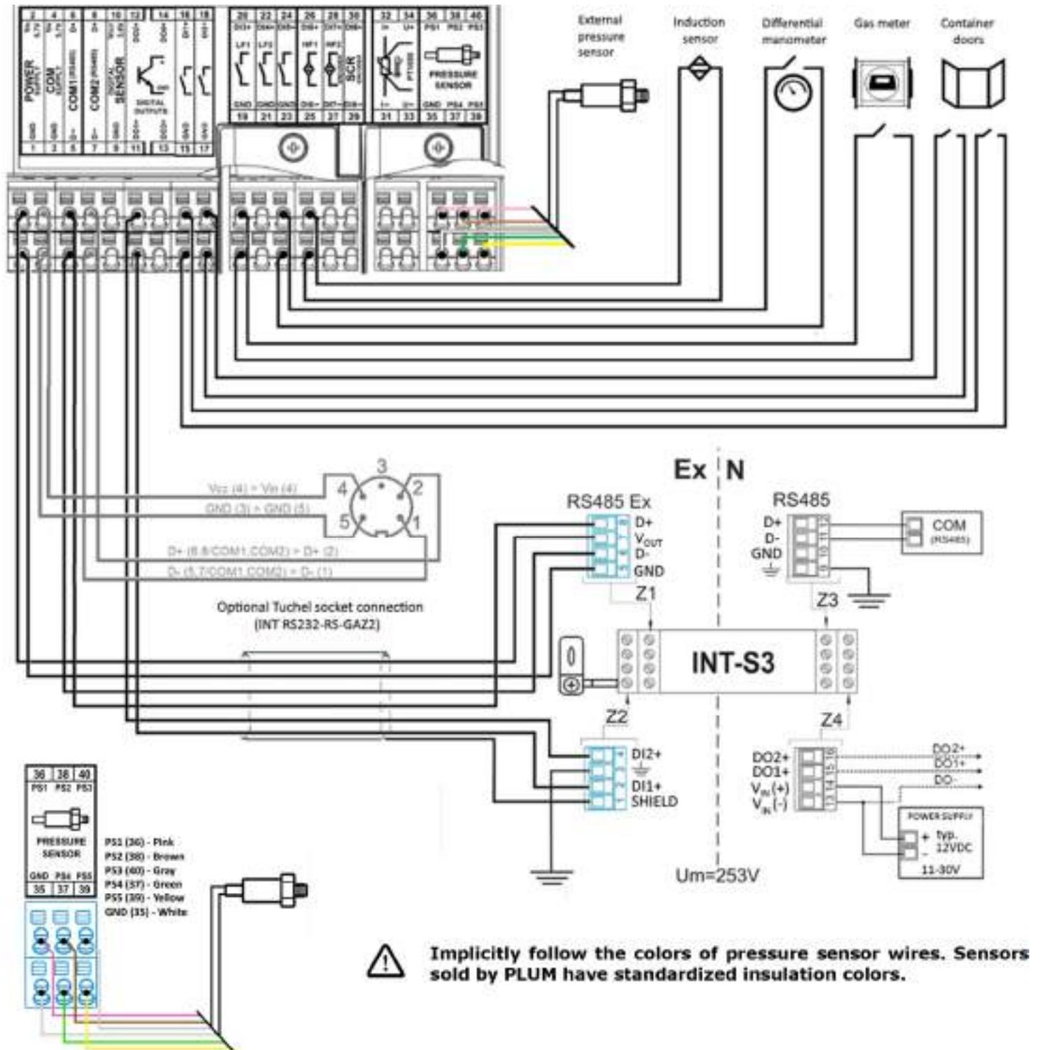
RS485Ex port in INT-S3 can be connected with COM1 or COM2 in MacBAT 5.
