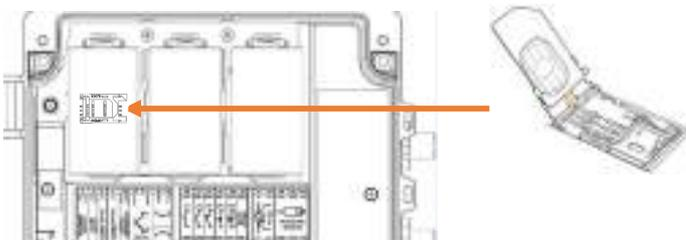
If the converter is equipped with internal modem a SIM card of miniSIM size must be placed inside, under the battery marked as B3. In place of one cable gland there is FME antenna socket to connect external mobile antenna. The antenna with the magnetic base should be fixed to a metal element nearby, such as the wall of a container.
