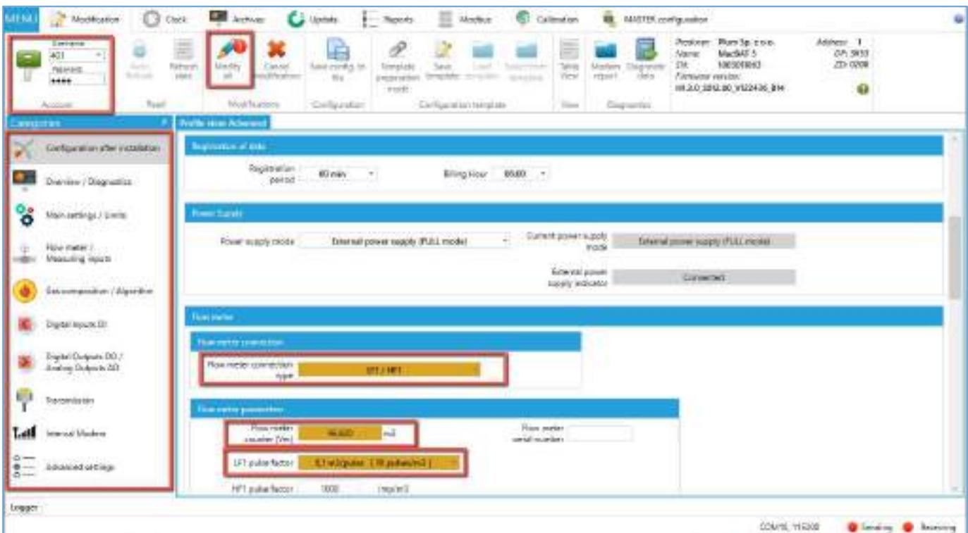
9. Set or choose authentication parameters (user name and password) in Account section, which allows device configuration. Application uses **401** account (Administrator) and **4096** password by default, to authorize modification of configuration.
