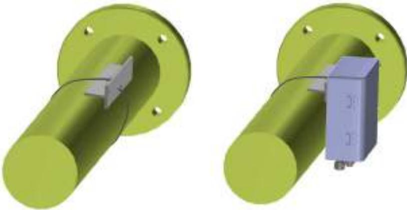
Select a suitable mounting location for the holder on the horizontal gas pipeline. Use a hose clamp to fix the holder to the gas pipe. Twist the clamp with a Phillips screwdriver to prevent the holder from moving on the pipe.
