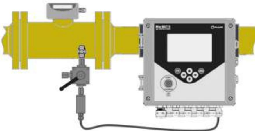
If the device is equipped with an external pressure sensor with the cable, it is not necessary to screw the three-way valve to the bracket itself. It is possible to locate the valve directly at the pressure gauge point, and sensor can be connected to the valve. There is no need for pulse tubes.
