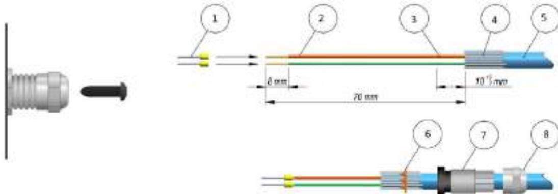
1 – ferrules, 2 – wires, 3 – foil, 4 – shield, 5 – cable, 6 – shaped gland ring, 7 – seal, 8 – gland nut.
