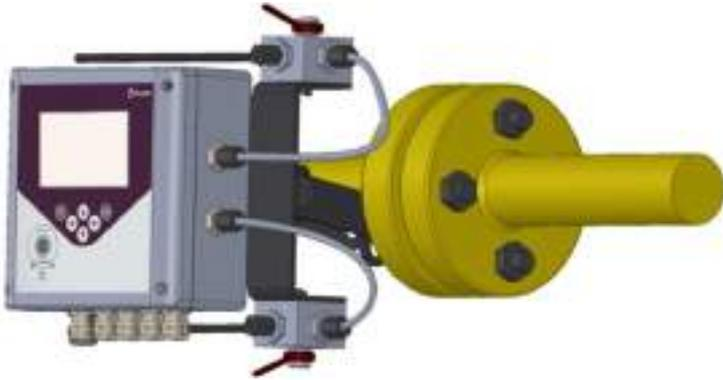
The bracket should be screwed under the one bolt that ties the pipe flanges together. Then, using the supplied M5x40 screws, tighten the device to the bracket. The mounting holes are accessible after opening the unit casing. Use the two holes on the right-hand side.
