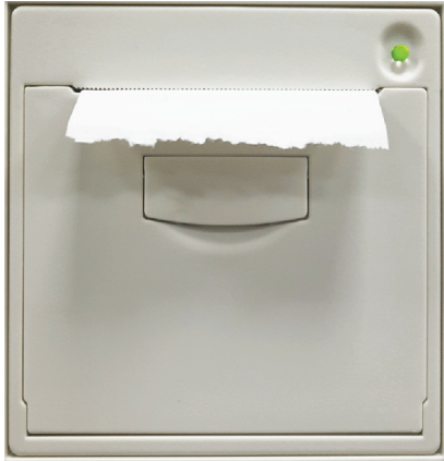
Figure 2-10 Installing Thermal Paper (3)
