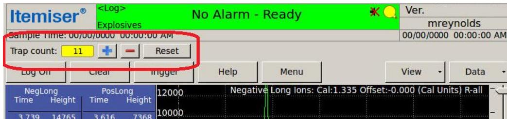
Each time you insert a trap into the desorber slot, the counter increases the number displayed by 1.
