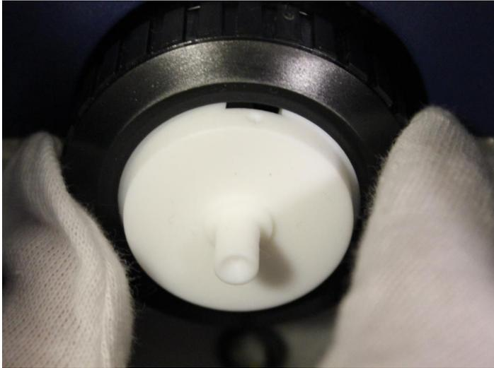
7. Remove the nozzle ring nut. Typically the nozzle comes off when you remove the nozzle ring nut. If it does not, gently pull it toward you and remove it from the device.
