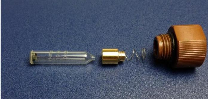
16. Verify that the O-ring on the lamp holder cap is undamaged and installed correctly.
