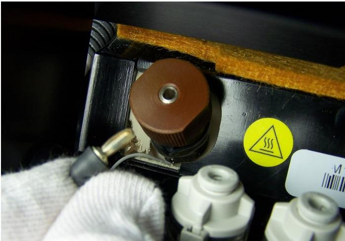
14. Close the side panel door and use the end of the lamp removal tool to latch the door (turn the tool 1/4 turn clockwise).
