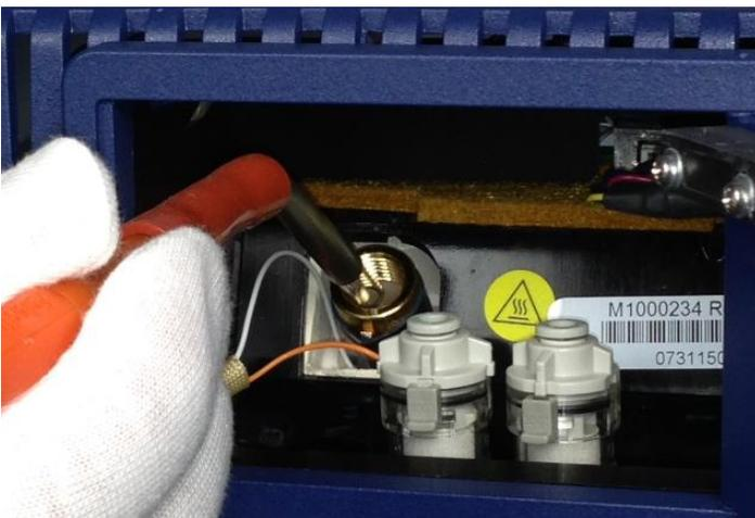
9. Remove the lamp from the end of the lamp removal tool. Note that you should not discard the lamp if you are required to generate an RMA.
