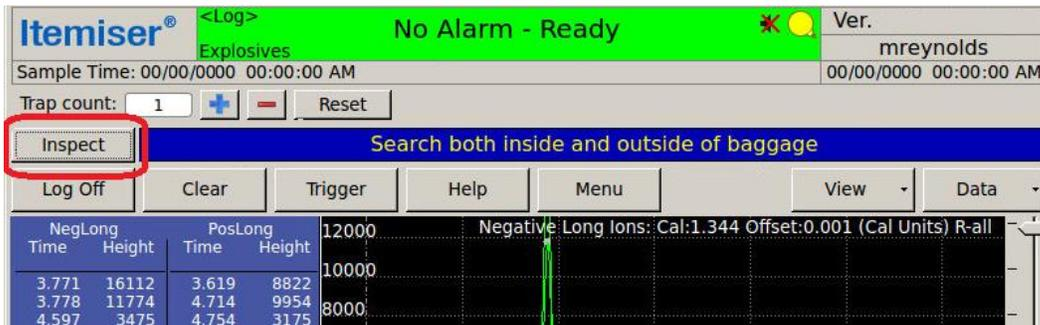
9. If you selected the *Change Search Type on every trigger* check box, then the device automatically changes the search type after each analysis of a sample trap.
