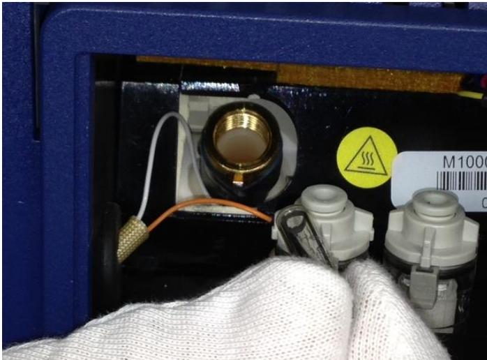
10. Install the lamp electrode-spring assembly into the lamp chamber; put the electrode (gold) end of the assembly in first.
