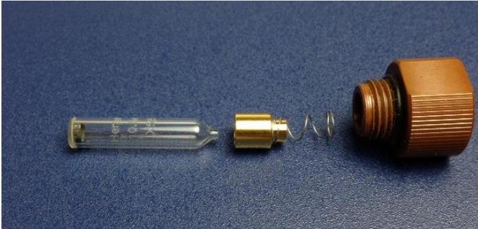
12. Screw the lamp holder cap clockwise onto the lamp chamber until the O-ring bottoms out on the chamber.
