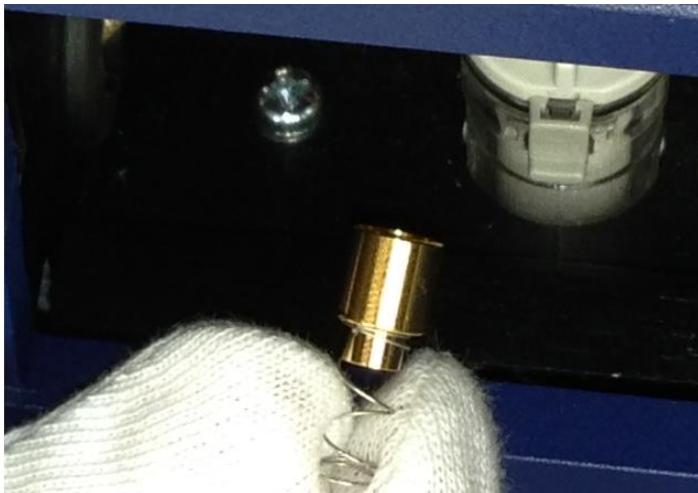
8. Insert the lamp removal tool onto the lamp and lift out the lamp.
