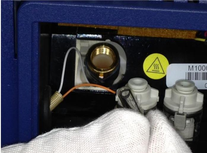
14. Install the lamp electrode-spring assembly into the lamp chamber; put the electrode (gold) end of the assembly in first.
