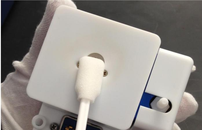
7. Install the desorber. Use the two alignment posts and make sure the connector is seated properly.
