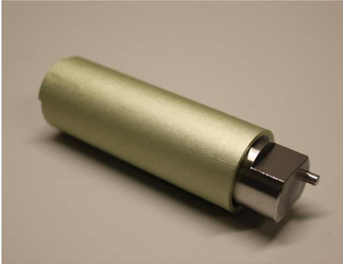
8. Push the calibrant end cap back in place. As you push the cap back into place, turn it slightly from side to side to make it easier to replace. Ensure that the cap is fully and securely installed.
