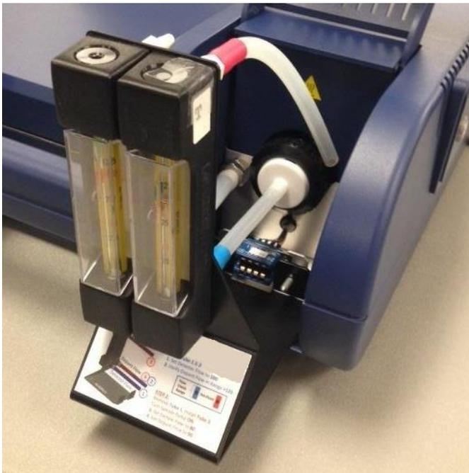
8. Ensure that you securely fit the two bottom tubes onto the device:
