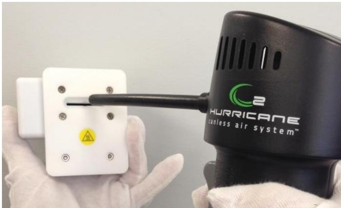
4. Blow out the hole in the rear of the desorber with several blasts of air.
