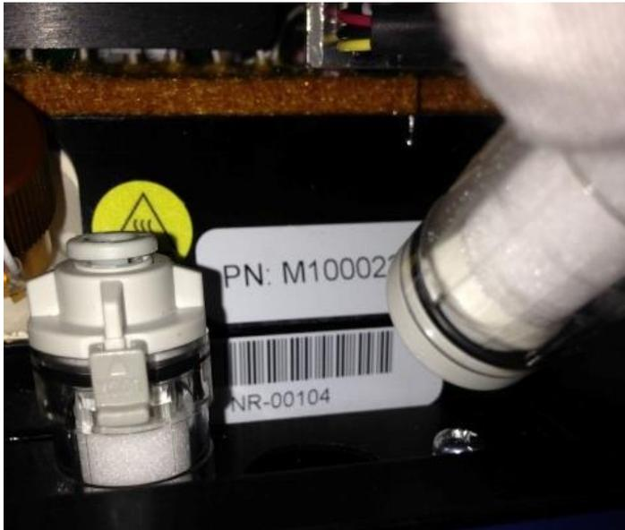
4. Push down on the gray latch to open the filter housing.
