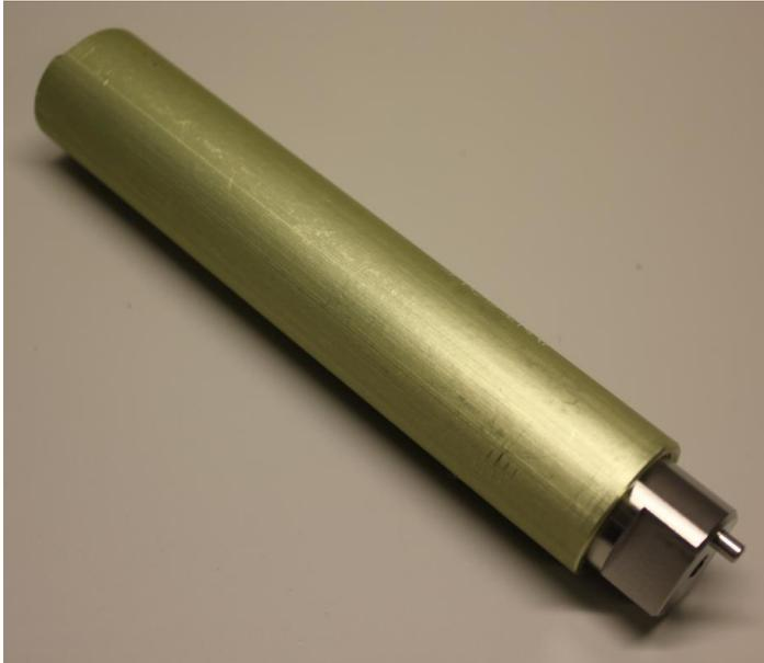
8. Push the negative (-) **DOPANT** end cap back in place. As you push the cap back into place, turn it slightly from side to side to make it easier to replace. Ensure that the cap is fully and securely installed.
