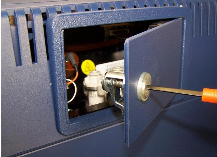
2. Check the color of both filters. Replace any filter that appears dirty (dirty filters appear brown or gray, while clean filters are white).
