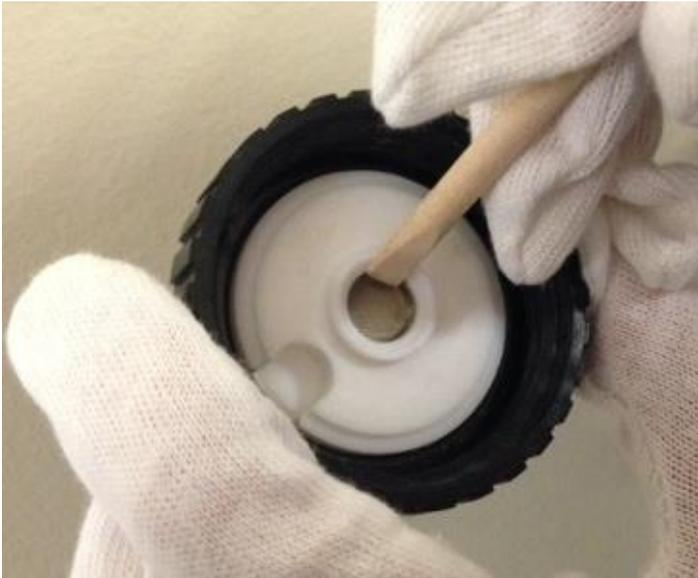
11. Put the nozzle ring nut onto the detector interface. Be sure the notch on the nozzle lines up with the pin on the detector interface.
