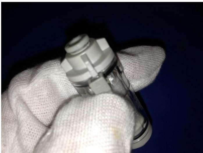
5. Remove the dirty filter and replace it with a new one.
