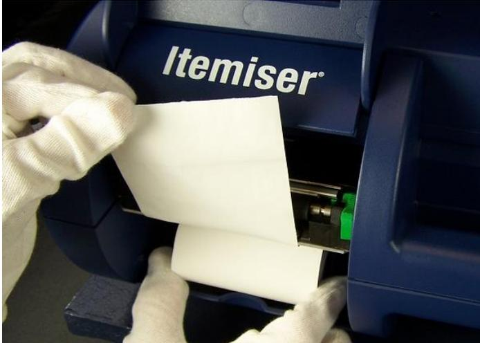
4. Push the bottom of the green lever to release the paper tension bar.
