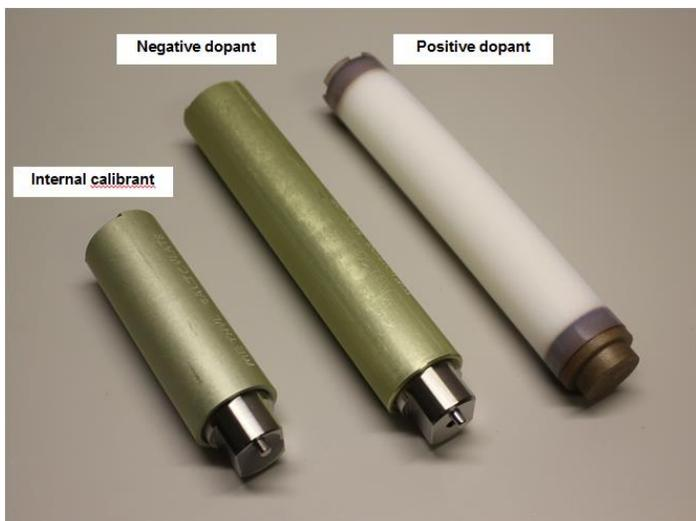
Whenever you install new dopant tubes, wait two hours before you attempt to use the device (this time is necessary for the dopants to diffuse into the device).
