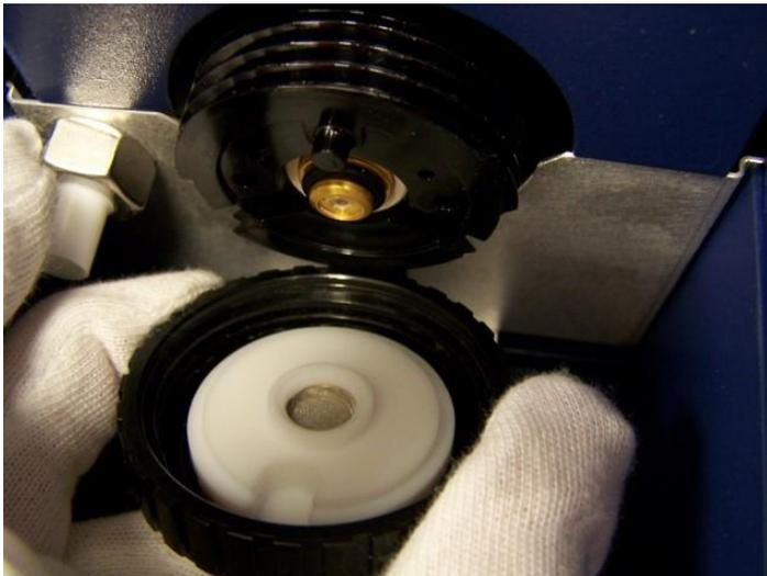
12. Tighten the nozzle ring nut until it is finger tight.
