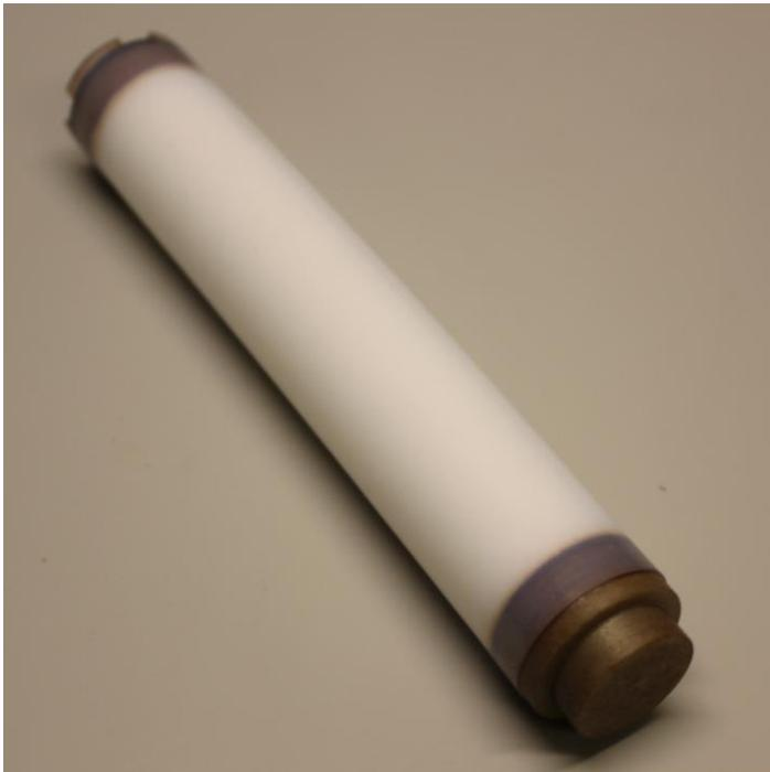
6. Visually inspect the substance level in the dopant tube.
