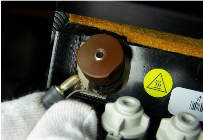
19. Close the side panel door and use the screwdriver end of the lamp removal tool to latch the door (turn the tool 1/4 turn clockwise).
