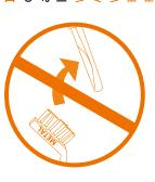
IMPORTANT: Do not use any metal objects to remove soiling from the acoustic waveguide as this may lead to scratches or other damage. WE RECOMMEND THAT YOU PREVENT ANY AND ALL CONTACT OF METAL OBJECTS WITH THE ACOUSTIC WAVEGUIDE (E.G. BLADES, CLIPS, TOUCHING GRASPING FORCEPS, ETC.).
