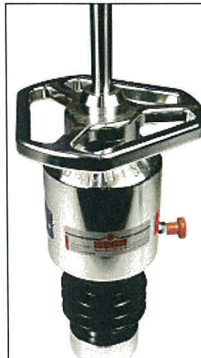
15 kg falling weight for an extended measuring range (Evd 70 - 105 MN/m 2 )
