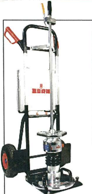
foldout trolley for easy ZFG transport between measurement points
