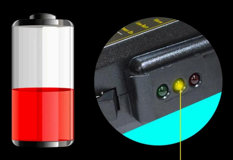
When the voltage is lower than 7V — Yellow low voltage indicator lights up
