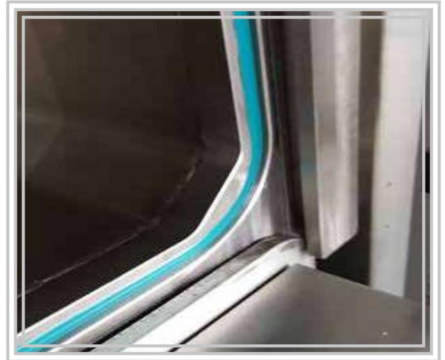
When the door is closed, there is a safety system that prevents any cistern squeeze and allows the door to move in the opposite direction. Pressure and vacuum sealing of the door is provided by silicon based seal which is resistant to the temperature of the device and door sealing is provided by applying vapor pressure to the gasket channel.
