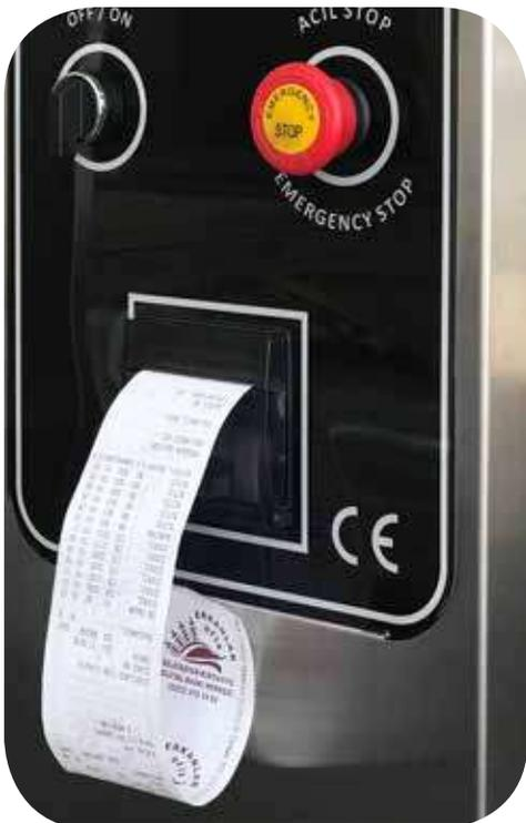
The thermal type printer located in the control unit is supplied with the following values as the cast:
