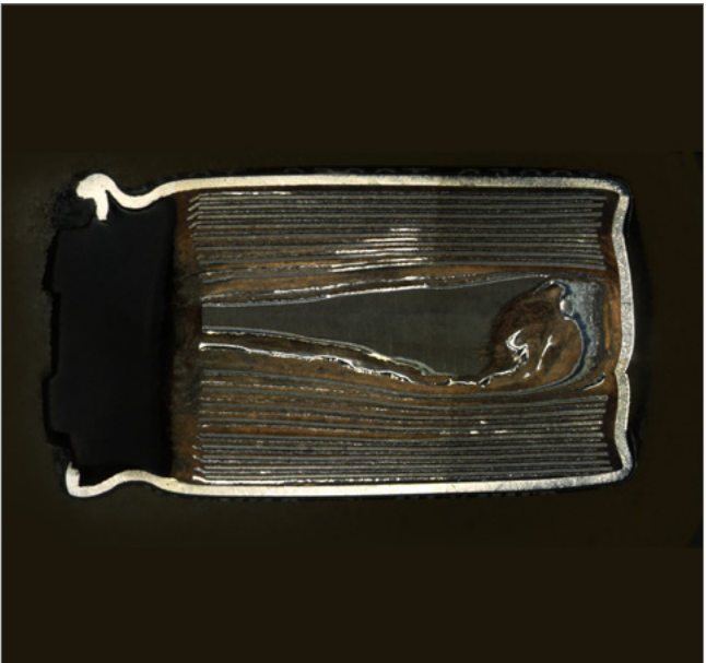
Foil capacitor, cut open, with dielectric in between; acquired with ZEISS Axio Zoom.V16, reproduction of object/camera 0.8
