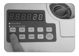
Press both Batch key and MEM key, then turn on the power, the machine will enter into the "batch changing mode" and the display show "bAt- SEt":
