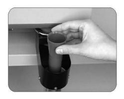
Put the Paper Tube into the Coin interior Tube and fall on the Coin Wrapper Stopper.
