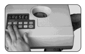
• Press <u>Batch</u> key to select the Memorized default batch quantities which you want to change; Change the selected default batch quantities by pressing +1000, +100, +10, +1 key.
