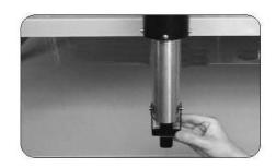
Select the Coin Interior Tube and Paper Tube according to the denomination of the counted coins.
