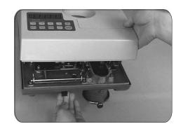
Then, pull up the Front Feed Pulley Arm and push & pull the Lock Plate upward to remove the foreign objects.(There is a diagram on the Side Cover to show how to open it.)
