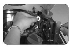
Restore the thickness adjustment Block and Front Feed Pulley Arm, close the Top Cover.
