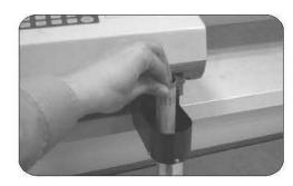
According to the coin quantity of each paper tube, select the batch quantity (in batch counting mode), then start counting. The machine will stop when the count total reaches the batch quantity. All the counted coins will drop into the Paper Tube, push the Coin Wrapper Stopper, backward, take out the Paper Tube and envelop it.
