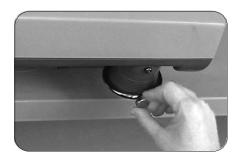
Attach the Coin Tube Holder, replace knob to lock into place.
