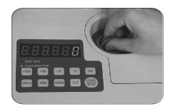
Set the Coin Thickness Adjusting Knob to the desired denomination according to the thickness of the coin.
