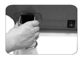
Put the coins into the Hopper and press the START/STOP key to start the counting. After the machine completes counting, all the small coins will be rejected into the Coin Reject Box or the Reject Coin bag.
