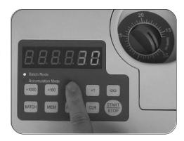
Press MEM key, save the amended default batch quantities in the memory, the previous default batch quantities will be replaced;
