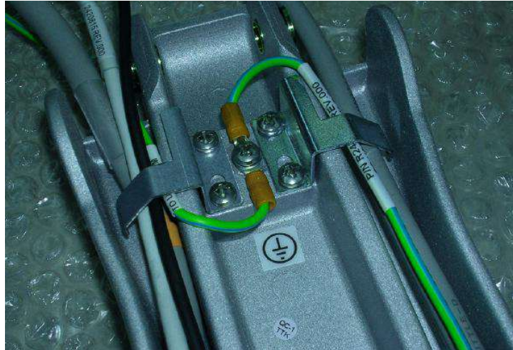
Figure 8-133 Positioning of Cable in Upper Arm
