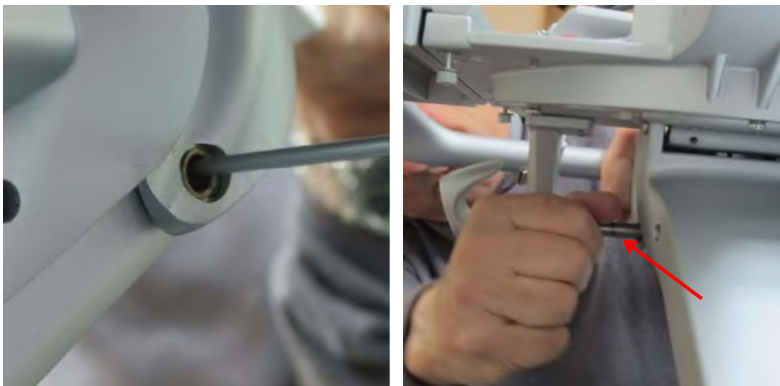
Figure 8-135 Remove Securing Pin
