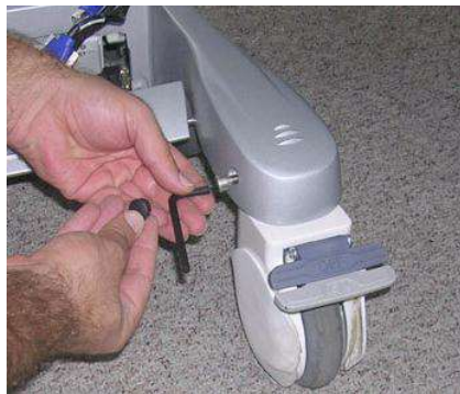
Figure 8-158 Removing the Securing Screw
