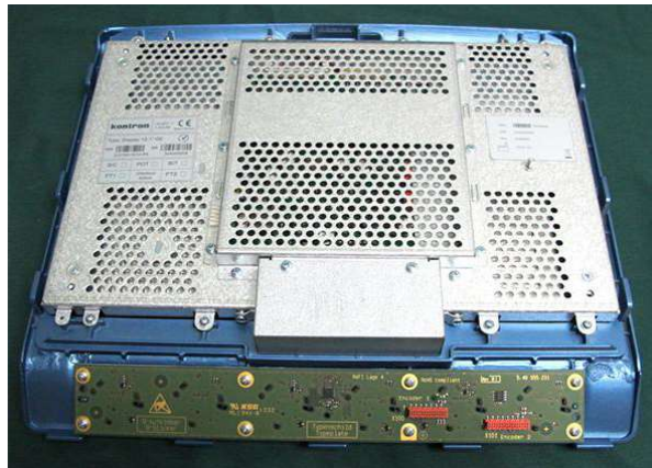
Figure 8-46 Touch Screen Removed
