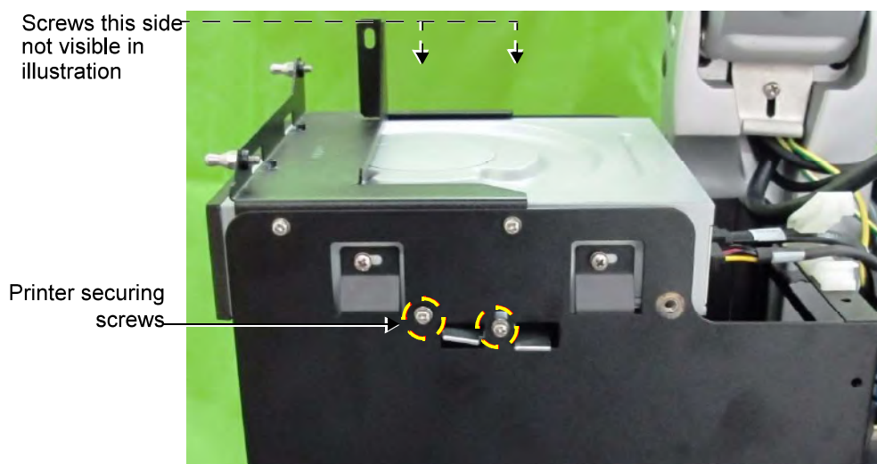
Figure 8-217 Screws Securing Black and White Printer in Compartment
