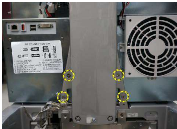
Figure 8-2. Install four screws at rear side
