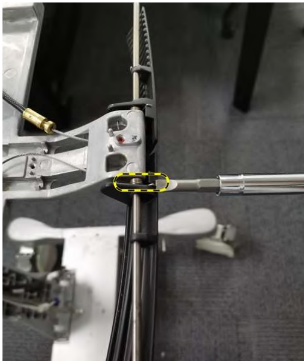
Figure 8-112 Release small spring hook
