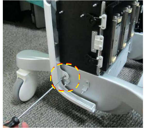
Figure 8-17 Right Rear Cover - Removing Securing Screws
