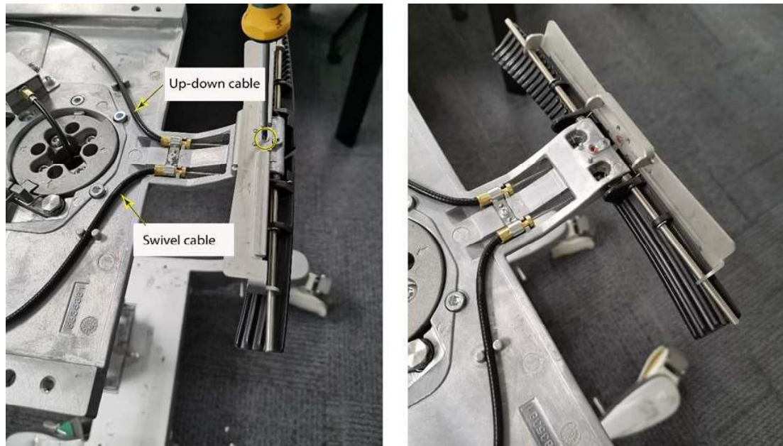
Figure 8-109 Protective Metal Plate Rotated 90 Degrees
