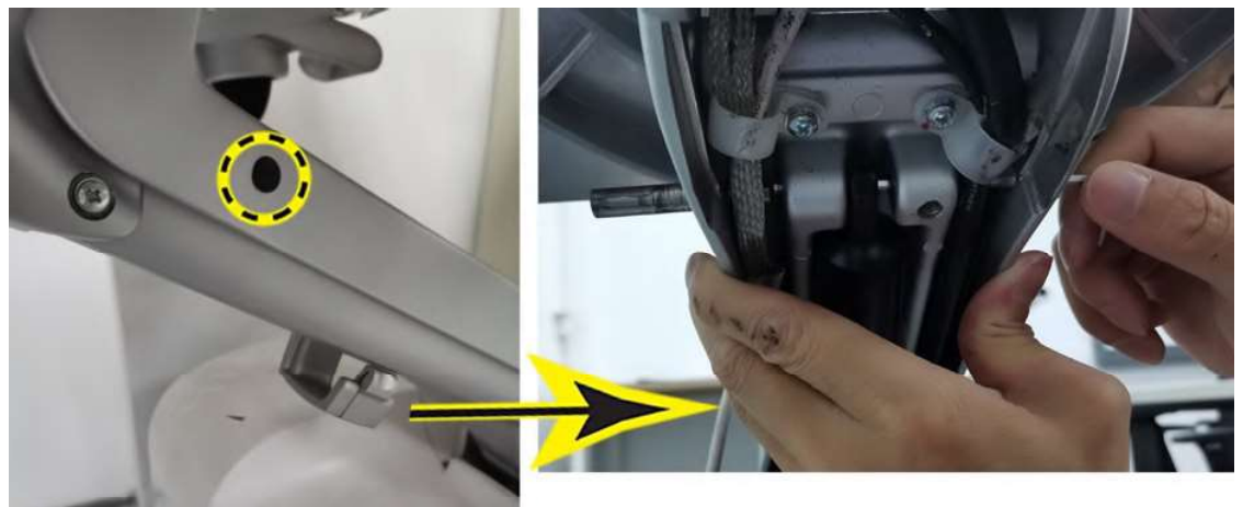
Figure 8-120 Remove screw covers and push out pins
