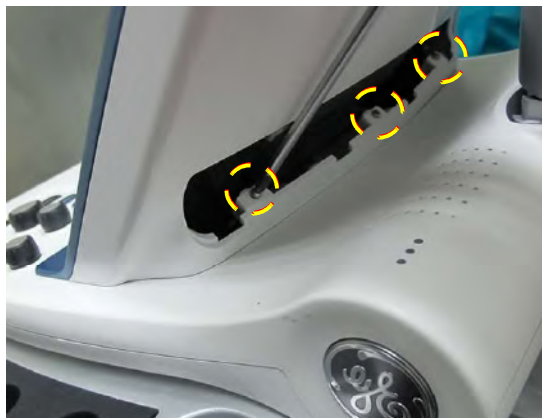
Figure 8-37 Removing the Rear Cover (Base) Securing Screws
