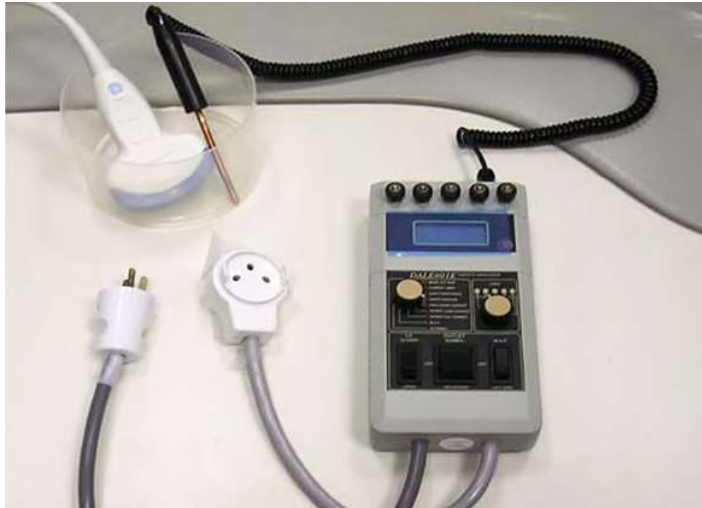
Figure 10-5 Test Set Up with Electrical Safety Analyzer
