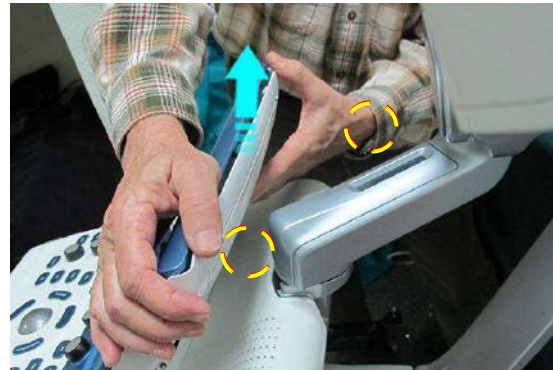
Figure 8-40 Removing the Touch Screen Securing Screws
