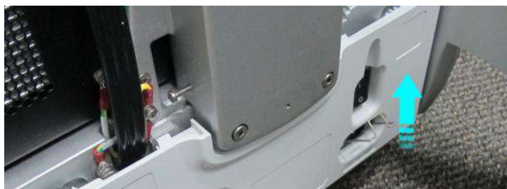
Figure 8-29 Removing the AC Distribution Box Cover
