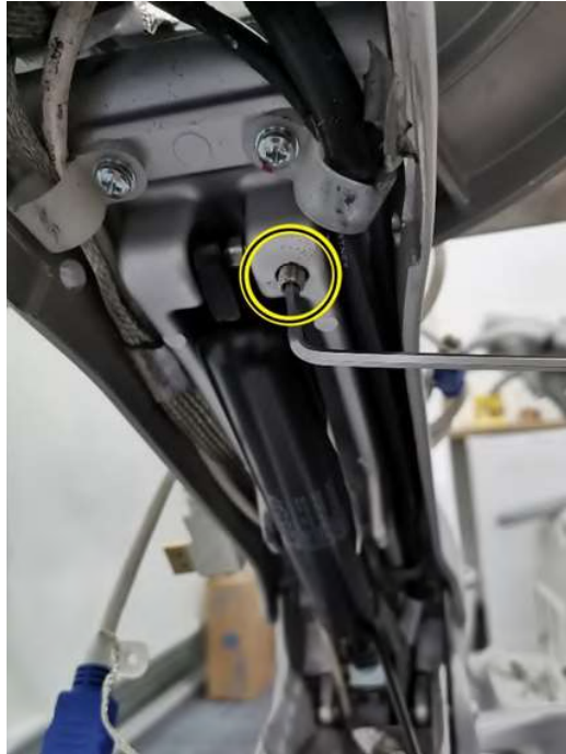
Figure 8-119 Remove screw from center
