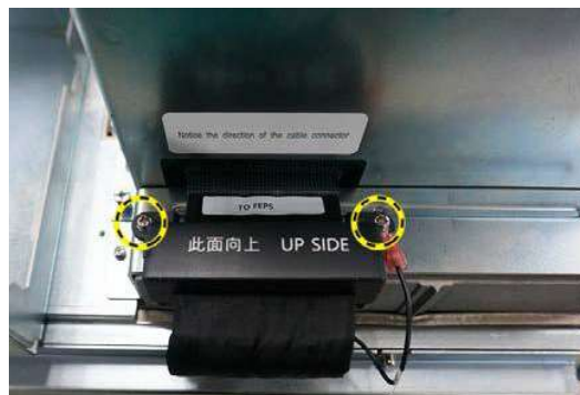
Figure 8-10. FEPS to CMST Cable
