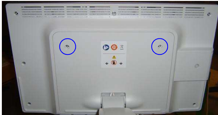
Figure 8-32 Monitor Rear Cover's fixing screws
