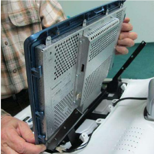
Figure 8-45 Removing the Touch Screen
