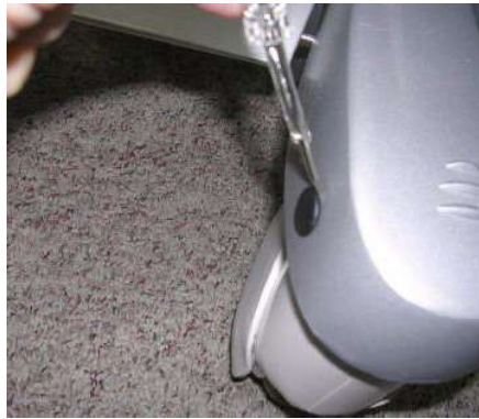
Figure 8-157 Removing the Screw Cap
