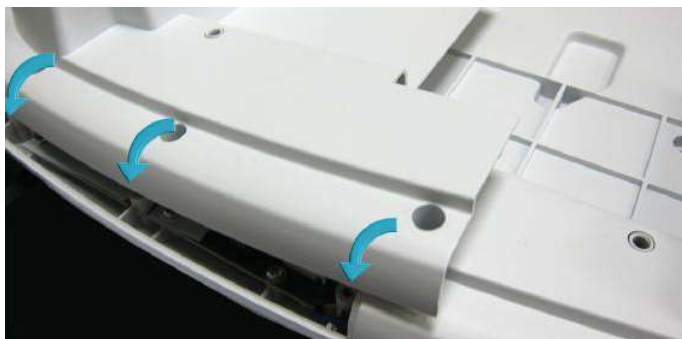
Figure 8-63 Fitting the Bottom Cover onto the Operating Panel Keyboard Assembly Base
