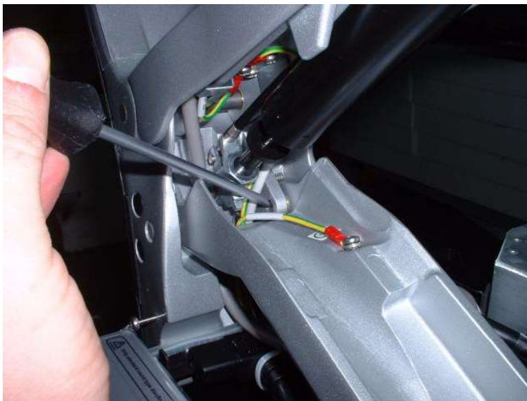
Figure 8-139 Removing Securing Pin and Disconnecting Ground Lead
