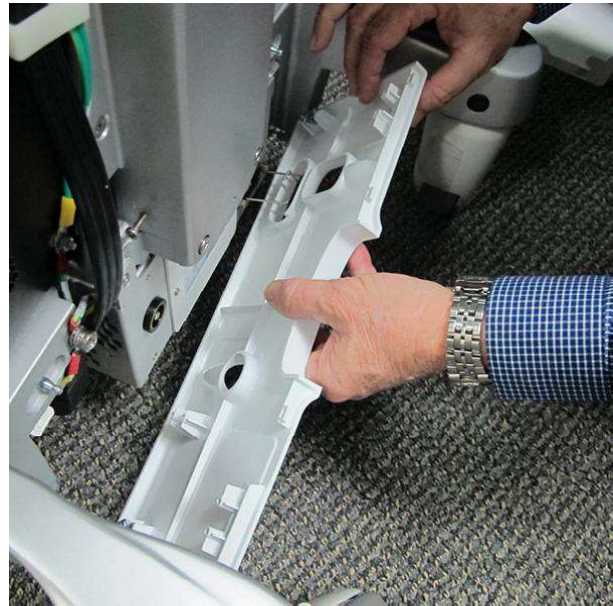
Figure 8-30 Removing the AC Distribution Box Cover
