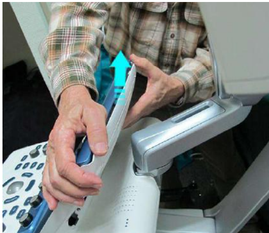
Figure 8-39 Removing the Touch Screen Rear Cover
