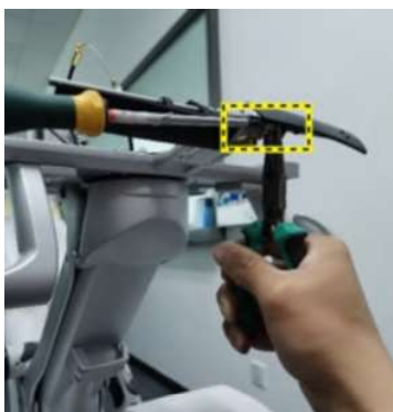
Figure 8-125 Stabilize the shaft and unscrew the cable
