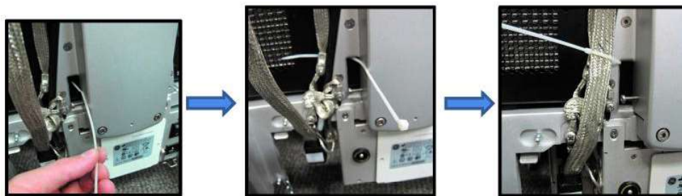
Figure 8-8. Add lower cable tie
