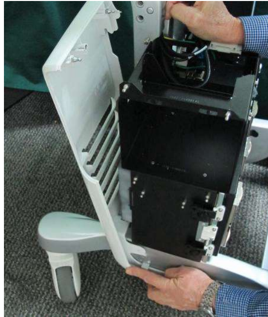
Figure 8-19 Removing the Right Rear Cover
