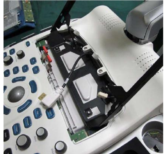
Figure 8-45 Removing the Touch Screen
