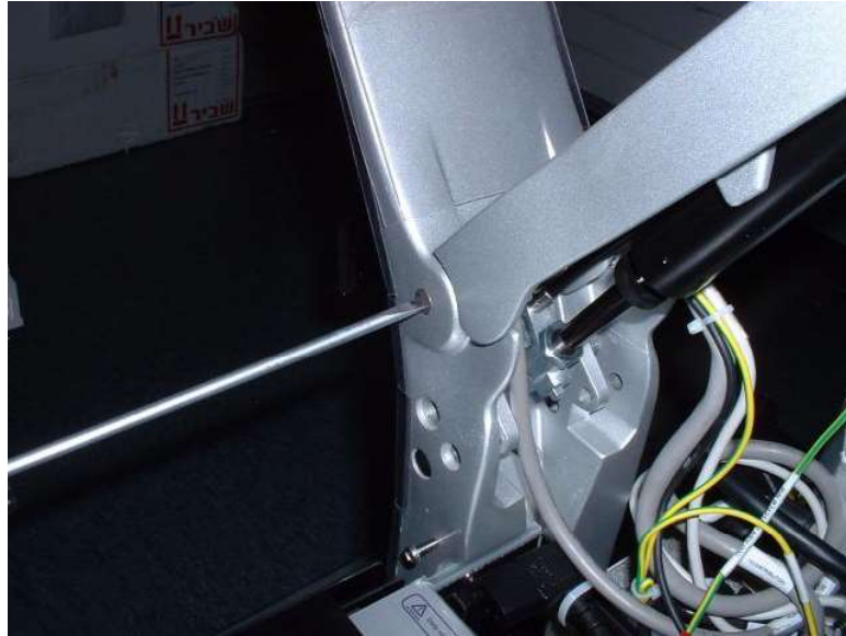
Figure 8-132 Tapping Out the Upper Arm Support Pin
