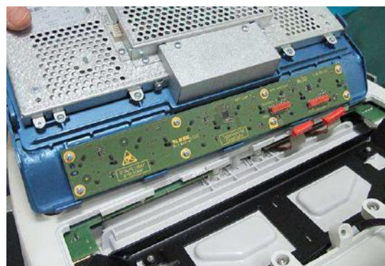
Figure 8-44 Disconnecting the Flex Cables
