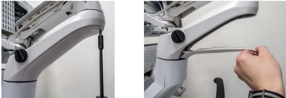
Figure 8-102 Remove the Lower Service Cover
