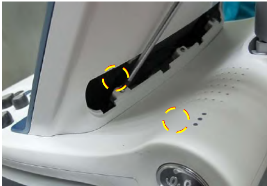
Figure 8-40 Removing the Touch Screen Securing Screws
