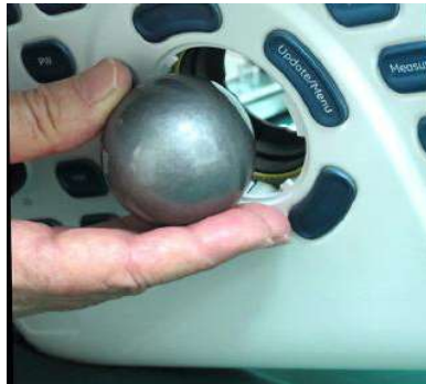
Figure 8-65 Removing the Mechanical Trackball
