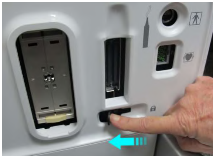
Figure 8-11 RS Probe Connector Lock - OPEN
