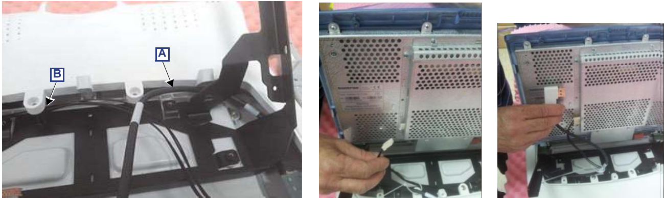
Figure 8-47 Routing and Connecting the Touch Screen Cables
