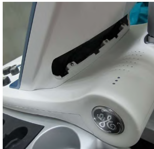
Figure 8-35 Removing the Touch Screen Service Cover
