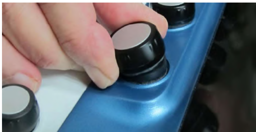
Figure 8-68 Removing a Rotary Knob
