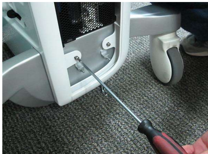
Figure 8-13 Removing Screw from Front Cover Securing Tab
