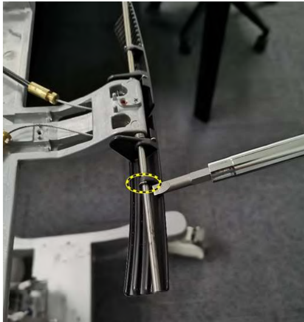
Figure 8-111 Remove spring clips
