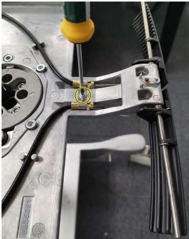
Figure 8-110 Unscrew cable clip
