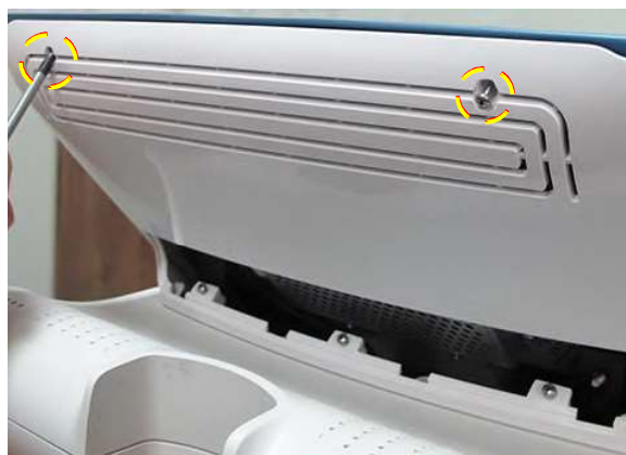
Figure 8-38 Removing the Rear Cover (Top) Securing Screws
