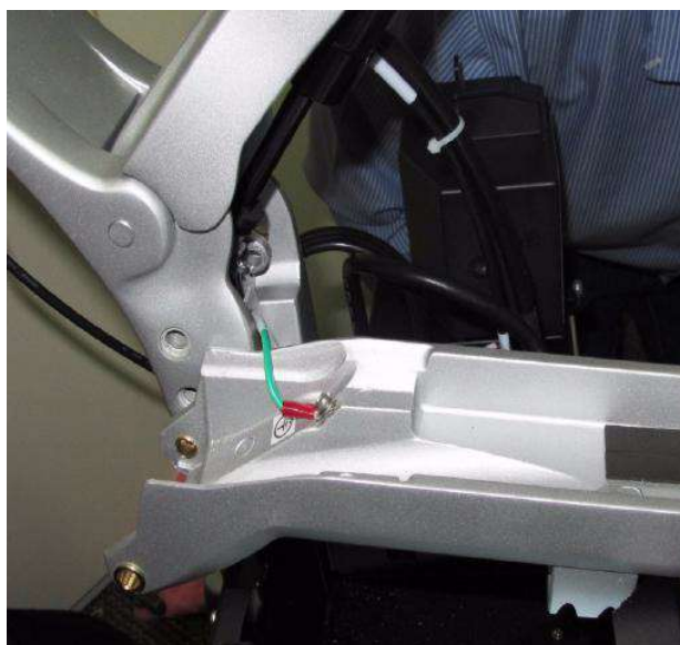
Figure 8-140 Removing the Lower Arm
