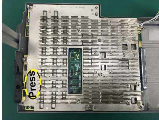
Figure 8-83 Press the CMST module
