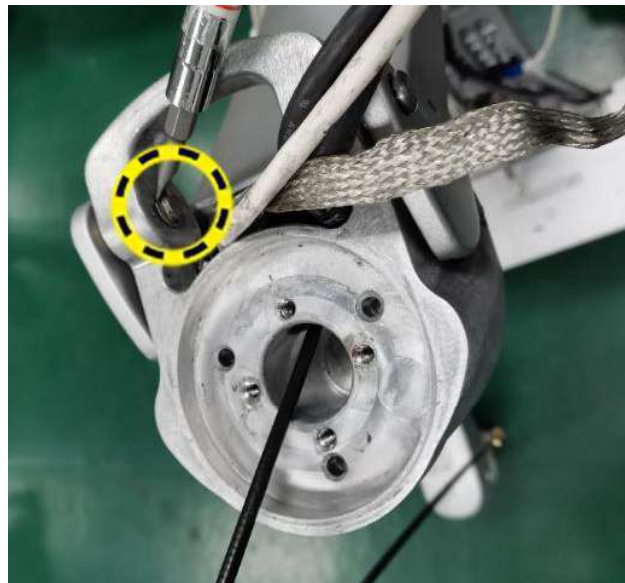
Figure 8-144 Ring Clips Securing Supporting Pins
