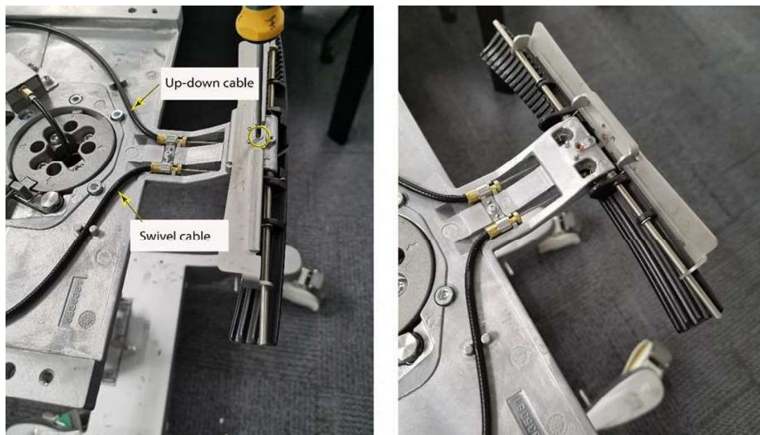
Figure 8-123 Protective Metal Plate Rotated 90 Degrees
