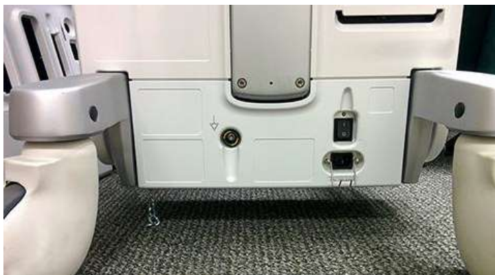
Figure 8-31 AC Distribution Box Cover Installed
