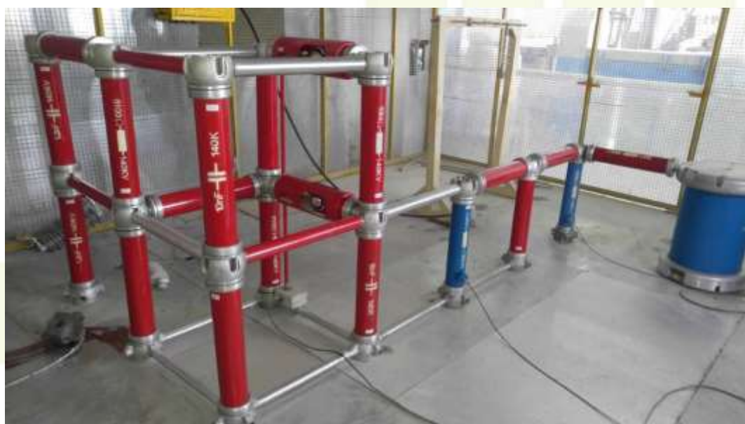
Figure 8: Equipment of Lightning Impulse Voltage Test
