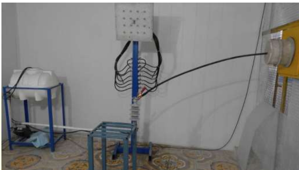
Figure 9: Wet Power Frequency Voltage Test Chamber
