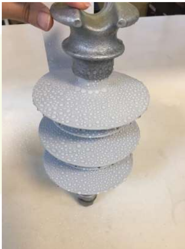
Figure 1: Hydrophobicity of the Insulator
