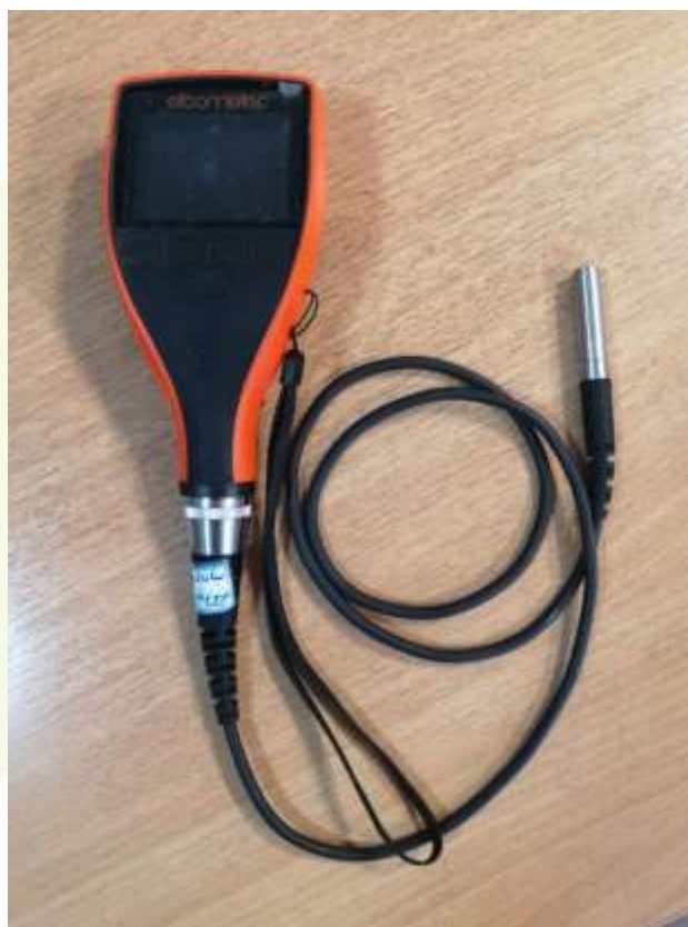
Figure 7: Equipment Used for Coating Thickness Measurement
