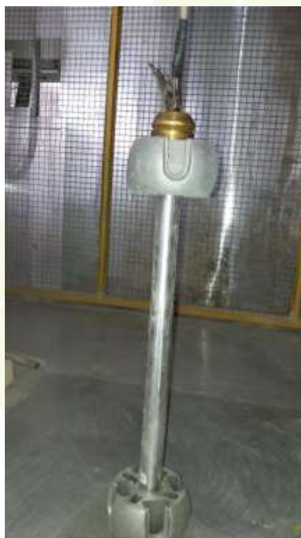
Figure 6: Brass Electrodes Used in Water Diffusion Test
