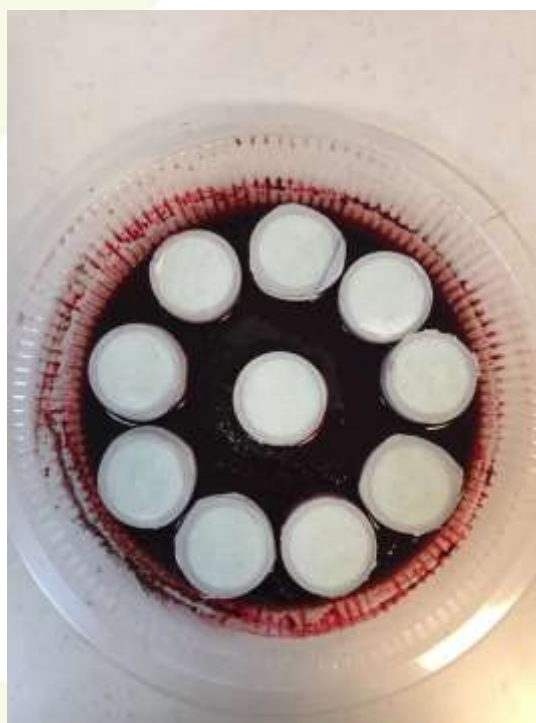
Figure 2: Schematic View of Dye Penetration Test
