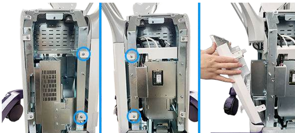
Figure 3-70 Remove the body back cover
