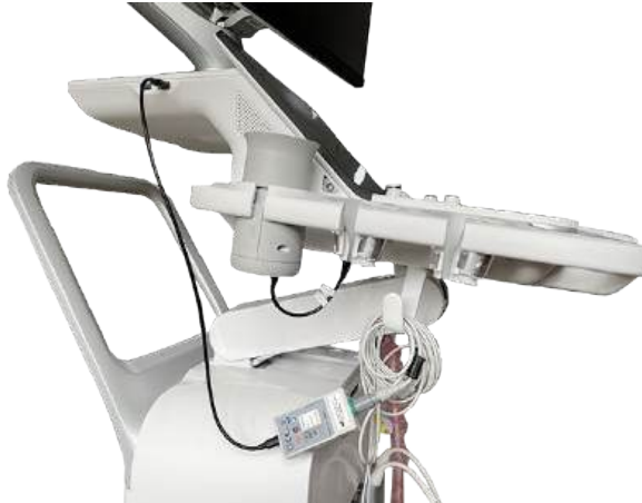
Figure 3-67 Connecting ECG to the system
