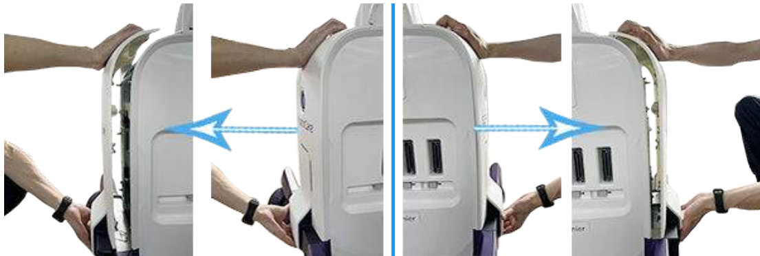
Figure 3-49 Remove body left and right cover
