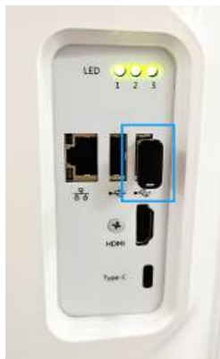
Figure 3-75 Connect Bluetooth Adapter
