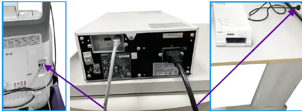
Figure 3-55 Color Printer connection
