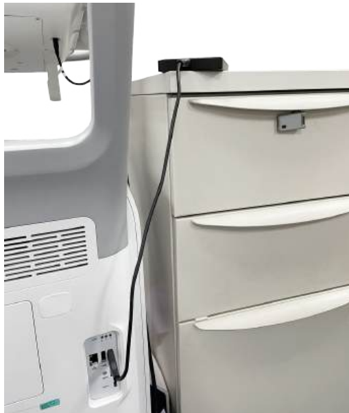
Figure 3-66 Connect HDD to the system
