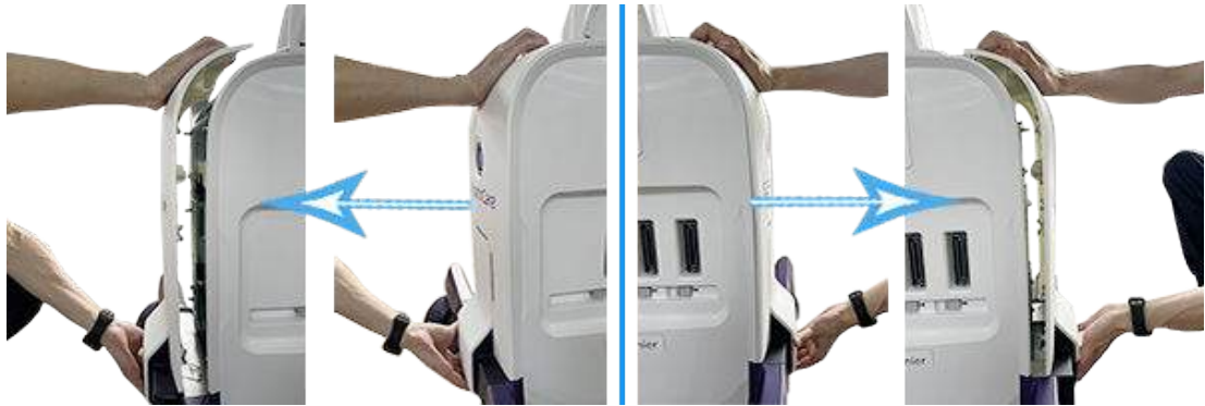
Figure 3-31 Remove the body front cover
