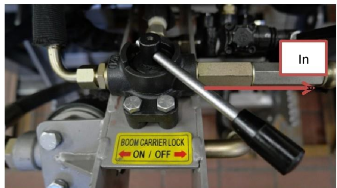
Fig.22 Hydraulic lateral displacement in
