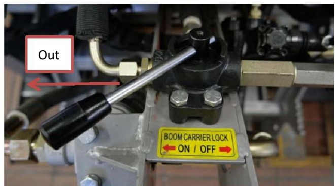
Fig.21 Hydraulic lateral displacement out
