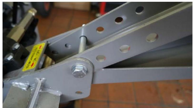
Fig.30 Partially assembled seat rods
