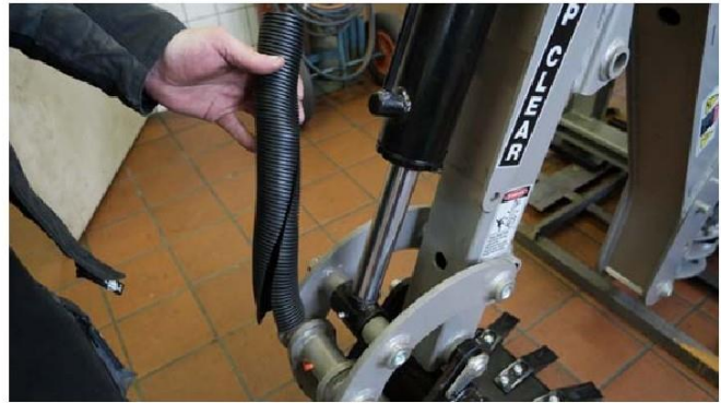
Fig.20 Removing the protective sleeves
