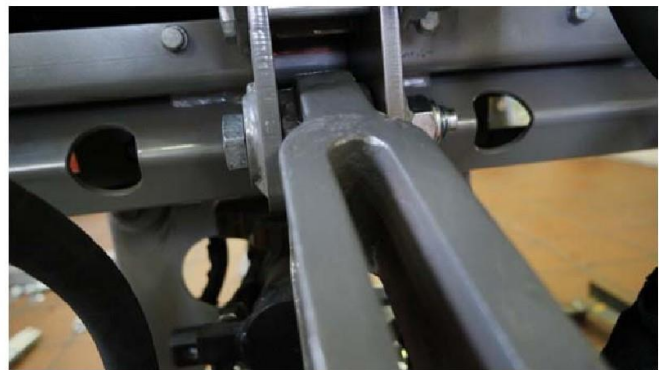
Fig. 48 Top link assembly on the digger
