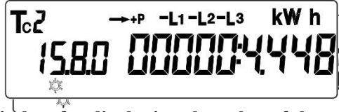
Figure 14. Window for displaying the value of the active energy module Figure 13. Window for displaying the current date on the clock 1/1/2000
