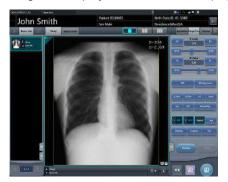
When the (2) work area zoom tab is pressed, the tool bar is hidden and the work area is enlarged. You can press the tab again to display the tool bar.
