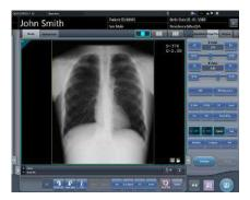
When the (1) work area zoom tab is pressed, the examination display area is hidden and the work area is enlarged. You can press the tab again to display the examination display area.
