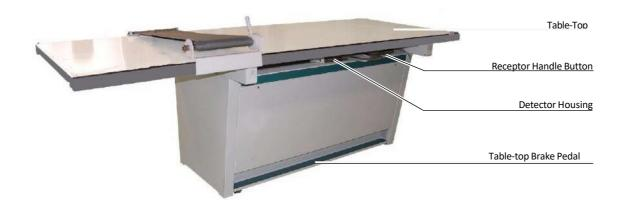
**TABLE-TOP BRAKE PEDAL**: The Table-Top is provided with a four-way floating movement for improved patient positioning. Pressing and maintaining the pedal down will release the longitudinal and transverse brakes of the Table-Top. Release the pedal to lock into position.
