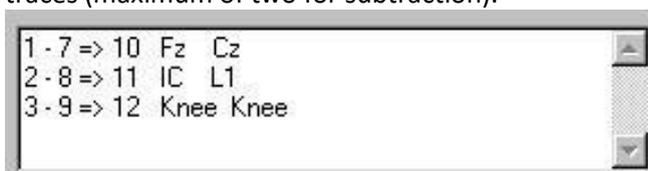
It is possible to work in a different way working on groups of traces that give as result a group of traces, each having the average data or the sum or the subtraction of the traces, each of every group taken
