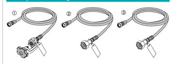
① A90121A Tubing "MAJ-1080", high pressure, for PIN gas cylinders ② A90122A Tubing "MAJ-1081", high pressure, for DIN gas cylinders 3 A90123A Tubing "MAJ-1082", high pressure, for ISO gas cylinders
