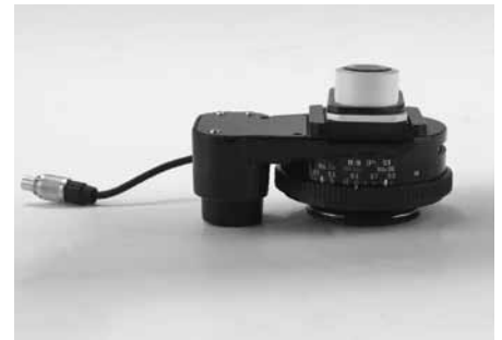
Fig. 16: Automated Condenser Achr. apl. A 0.9 (P) (only with Leica DM3000)
