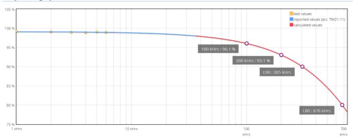
$\it LxB50$  results according to  $\it LM-80$  and  $\it TM-21-11$  procedures and norms.
