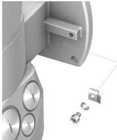
Figure 42: Earth connection for wall bracket
