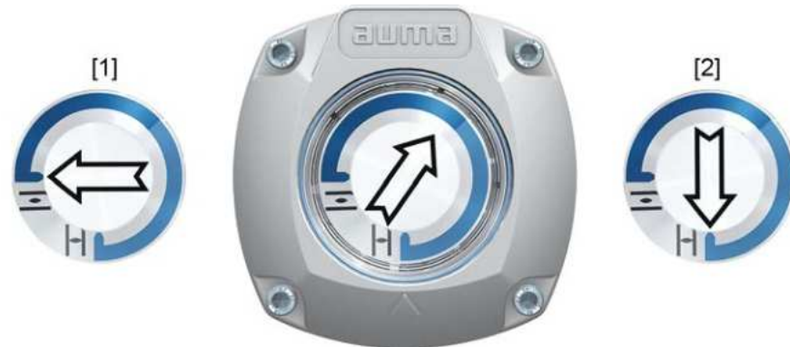
Figure 75: Mechanical position indicator
