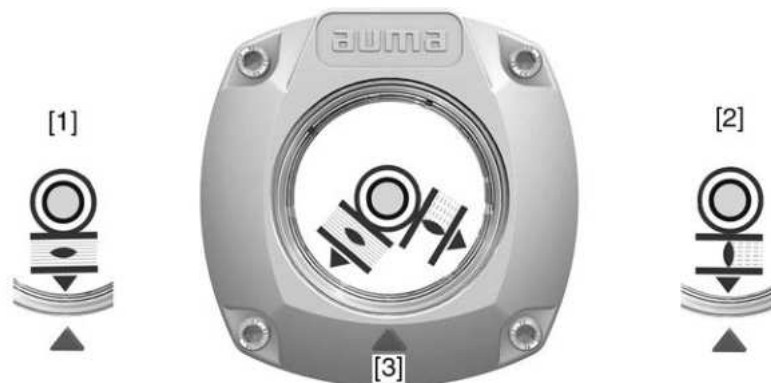
Figure 76: Mechanical position indicator
