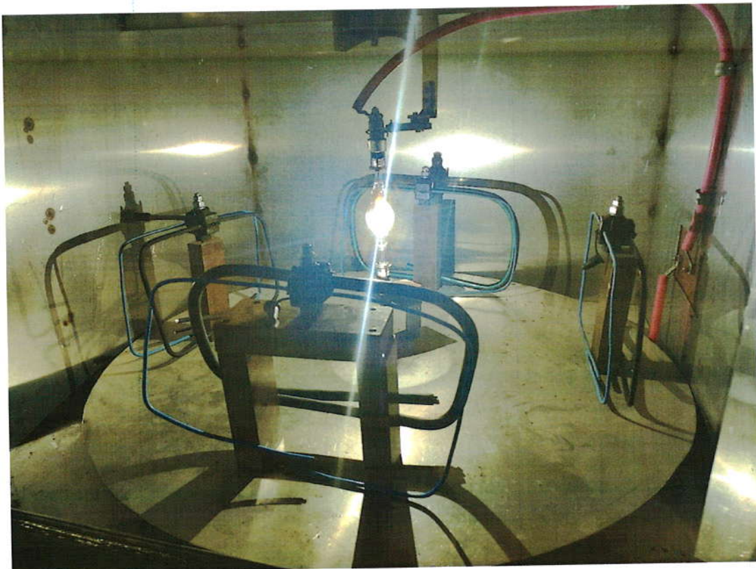
Fig.2 – IPC during the testing in the solar radiation simulation chamber
