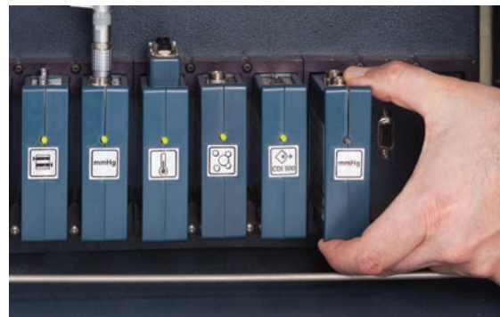
The Terumo System 1 can integrate up to 18 modules. These compact modules are plugged into the base of the system.
