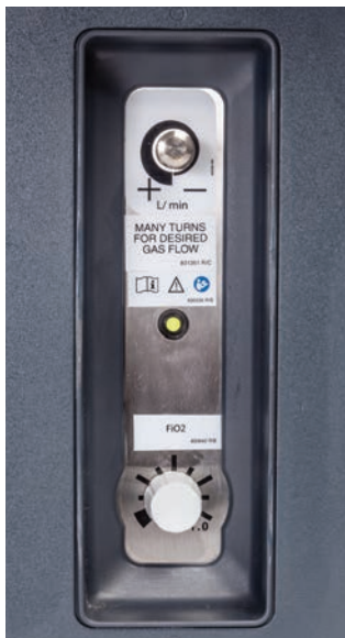
Integrated electronic gas blender can be controlled through the Central Control Monitor or locally.
