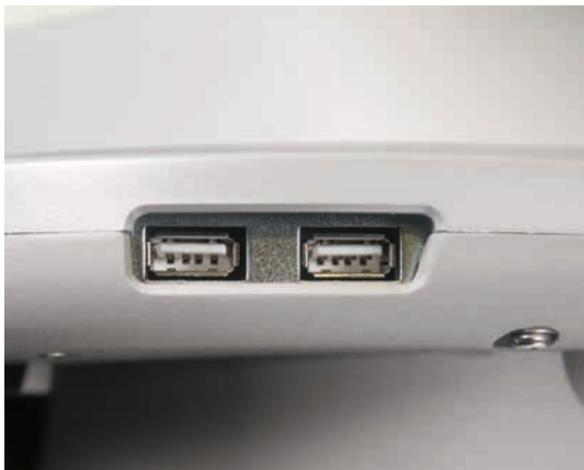
Two **USB ports** are also located on the back of the control panel.
