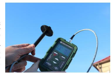
Measurement of coatings non-ferrous metals – the NF-2 sensor is used at measurements from 0 to 2 mm (2000  $\mu$ m).
