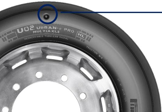
Patent **median groove shapes** design (Prometeon Patent) keeps constant the grip during all tyre life and improving the wet handling.
