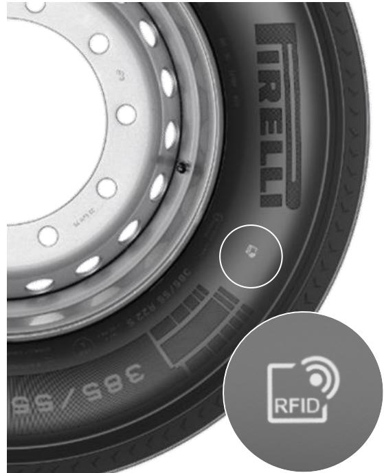
**RFID** chip is a smart electronic component that receives and transmits radio signals (without cables). It is incorporated inside the tire and allows for simple identification and easy connection to tire management and tracking systems. RFID contains ISO-encoded unique tyre identification according to the SGTIN96 standard.
