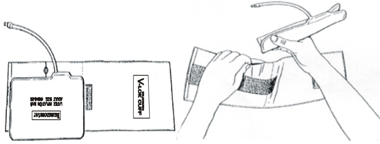
Fig 24-1 Replacement of Rubber Tube in the Cuff
