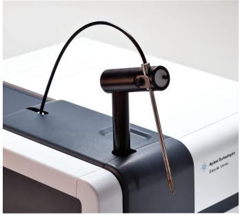
**Eliminate cuvette and sipper hassles**By using fiber optics probes, you'll never have to buy or clean a cuvette again.
