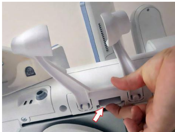
Figure 2-10 Removal of the left and right Endocavity probe holders. For installation, just push them back into the user interface until you hear a "click" noise.
