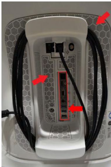
Figure 2-5 Air filters and the connector area at the back of the system.
