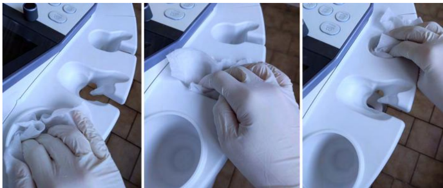
Figure 2-7 Cleaning and disinfection of the left and right Probe and Gel Holders. Repeat with shown procedure on the whole part (top and bottom, each holder separately)
