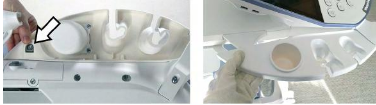
Figure 2-8 Removal of the basic version of the left and right Probe Holder inserts. For installation, just push them back on the user interface until you hear a "click" noise.
