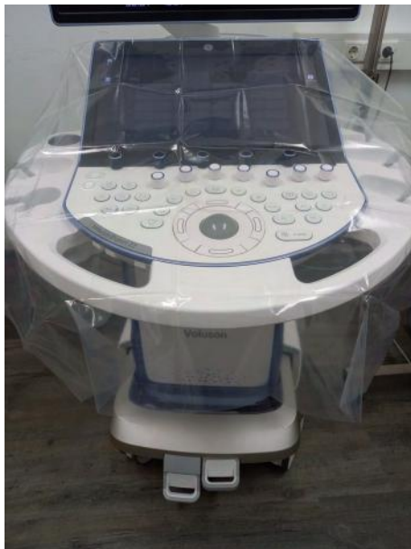
Figure 2-6 Sterile system drape for User Interface of the Ultrasound console (e.g., CIVCO - part number 610-02)
