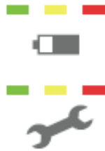
Figure 2. Back-up panel battery and maintenance LED indicators
