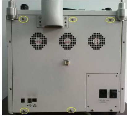
Figure 3-5 Host Rear Cabinet Installation
