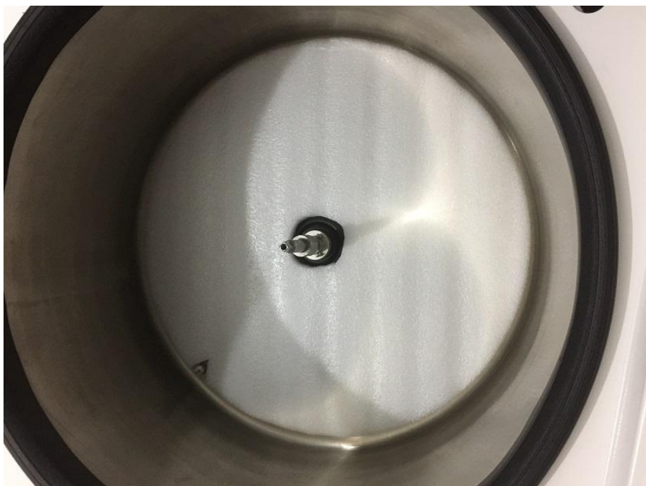
Padding between rotor bowl and chamber
