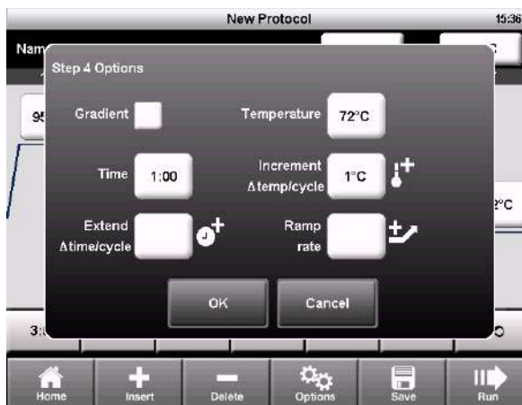
Figure 12. Step 4 has a temperature increment option.
