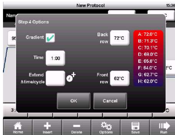
Figure 10. The Step Options window displays the gradient temperatures.
