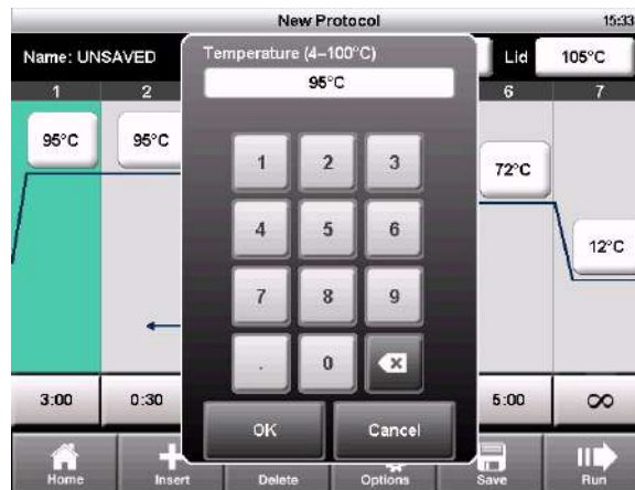
Figure 7. Editing a temperature with the numeric keypad.
