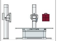
Floor-mounted solution with manual Bucky wall stand and fixed table equipped with Core XL for free exams
