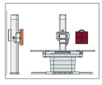
Floor-mounted solution with motorized Bucky wall stand with Core static and elevating table equipped with Core XL for free exams
